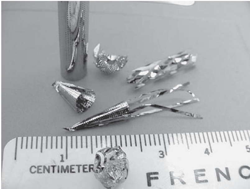
Figure 3.10 Photograph of cylinders, cones and other shapes made by the multiple-layer deposition method.
