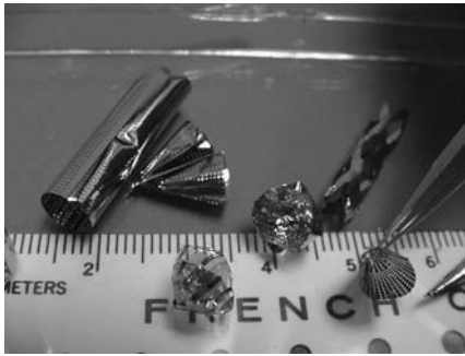
Figure 10.7 Photograph showing a variety of three-dimensional devices formed from sputtered thin film TiNi. Sizes can range from less than a millimeter to several centimeters. Stiffness depends on film thickness—thin films are very flexible and can be folded for implantation by a microcatheter. Photolithography provides a versatile means for fenestration of thin films.
