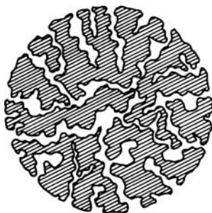
Figure 2.5 Pore structure of a stationary phase particle.
