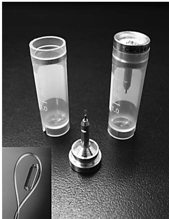
FIGURE 7.6 The standard copper pin used to mount protein crystals for data collection under cryoconditions. At the top of the pin, seen magnified in the inset, is a small fiber loop of 0.1 to 0.5 mm diameter that is used to “catch” or “scoop up” the crystal from its mother liquor. The magnetic base attaches to the goniostat. Also shown are cryovials where pins carrying crystals can be inserted for protection during storage in liquid nitrogen. (Courtesy of Hampton Research.)
