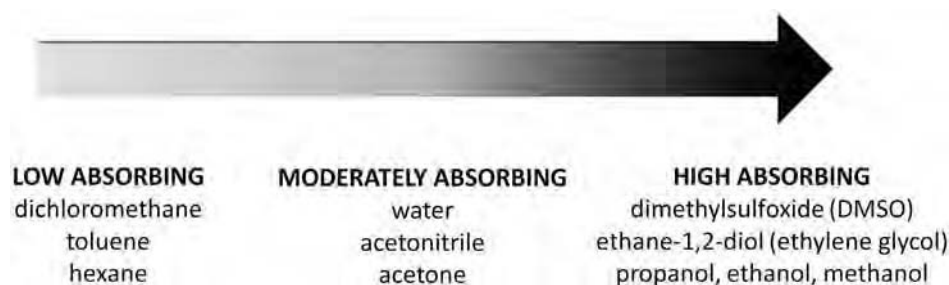
Figure 3.23 The heating characteristics of common solvents.
