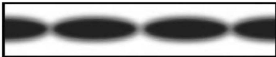
Figure 3.24 Areas of high and low microwave energy are found in the cavity of a multimode microwave unit.
