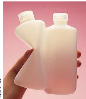
Figure 23.1 Branched and linear polyethylene. The polyethylene bottle at the left is made of pliable, branched polyethylene. The one at the right is made of semirigid, linear polyethylene.
