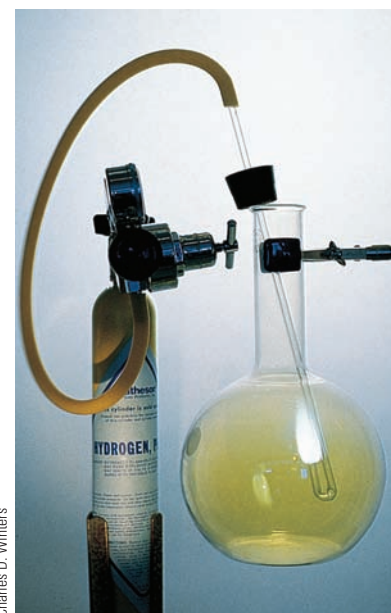
An exothermic reaction. Hydrogen, a colorless gas, reacts with chlorine, a pale yellow gas, to form colorless hydrogen chloride gas.
