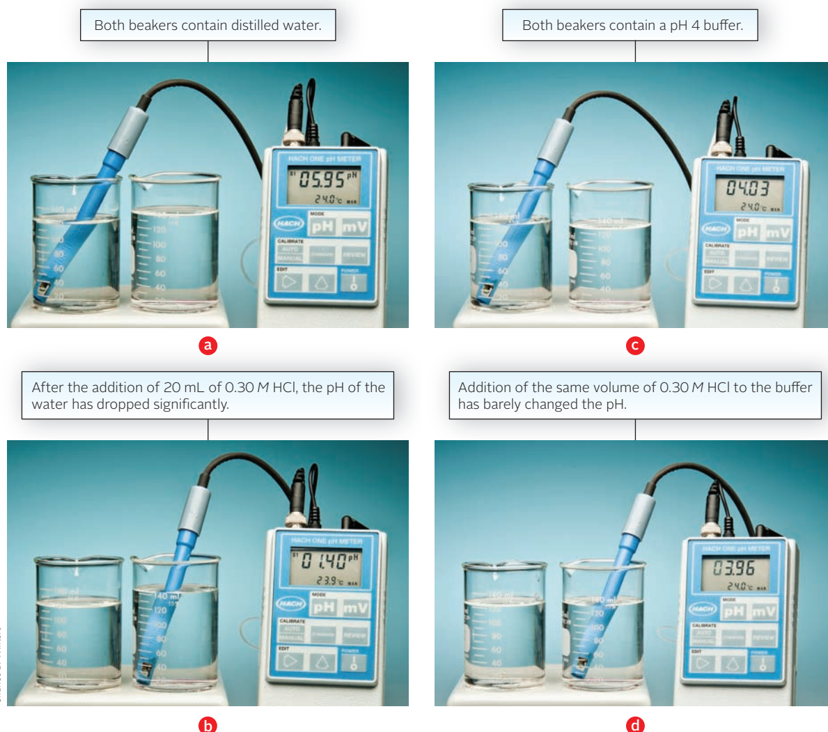
Figure 14.1 The effect of a buffer upon addition of acid. Note the reading on the pH meter.
