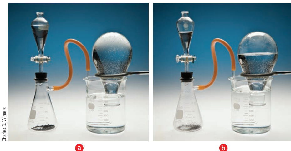
Figure 5.7 Collecting a gas by water displacement. (a) Hydrogen gas is being generated in the flask by an acidic solution dripping onto a metal. (b) When a gas is collected by displacing water, it becomes saturated with water vapor. The partial pressure of \text{H}_2\text{O}(g) in the collecting flask is equal to the vapor pressure of liquid water at the temperature of the system.
