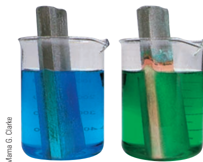
Figure 17.5 Oxidation of Ni by \text{Cu}^{2+} . Nickel metal reacts spontaneously with \text{Cu}^{2+} ions, producing Cu metal and \text{Ni}^{2+} ions. Copper plates out on the surface of the nickel, and the blue color of \text{Cu}^{2+} is replaced by the green color of \text{Ni}^{2+} .
