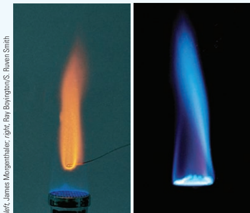
Figure C Flame tests for \text{Na}^+ (yellow) and \text{K}^+ (violet). A drop of solution is picked up on a platinum loop and immersed in the flame. The test for \text{K}^+ is best done with a filter that hides the strong \text{Na}^+ color.
