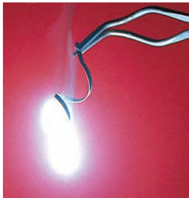
Figure 20.7 Burning magnesium. A piece of magnesium ribbon bursts into flame when heated in the air; the product of the reaction is \text{MgO}(s) .
