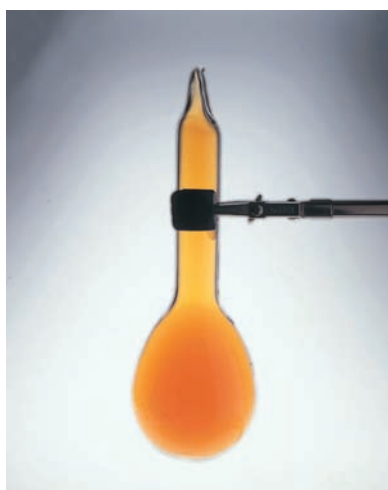
Nitrogen dioxide (NO 2 ), a binary molecular compound. It is a red-dish-brown gas at 25°C and 1 atm.
