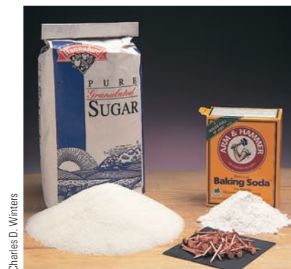
Figure 3.1 One-mole quantities of sugar (C 12 H 22 O 11 ), baking soda (NaHCO 3 ), and copper nails (Cu).
