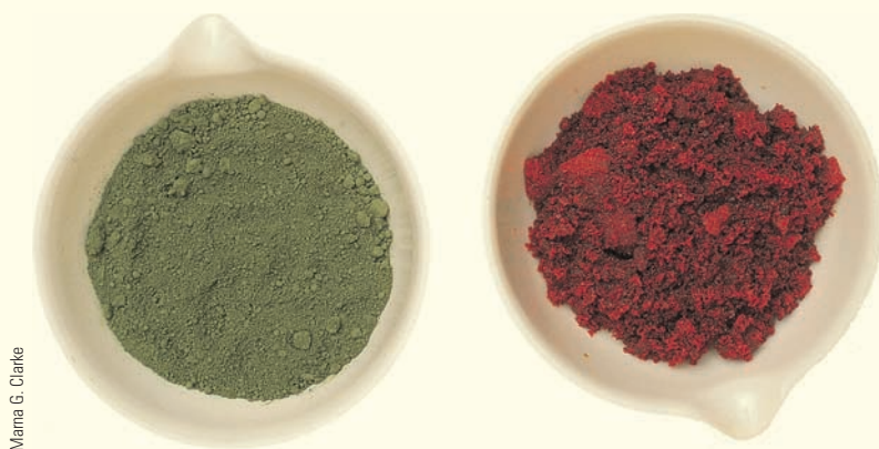
Figure A Chromium-oxygen compounds and the law of multiple proportions. Chromium forms two different compounds with oxygen, as shown by their different colors. In the green compound on the left, there are two chromium atoms for every three oxygen atoms ( 2\text{Cr}:3\text{O} ) and 2.167 g of chromium per gram of oxygen. In the red compound on the right there is one chromium atom for every three oxygen atoms ( 1\text{Cr}:3\text{O} ) and 1.083 g of chromium per gram of oxygen. The ratio of the chromium masses, 2.167:1.083, is that of two small whole numbers, 2.167:1.083 = 2:1 , an illustration of the law of multiple proportions.
