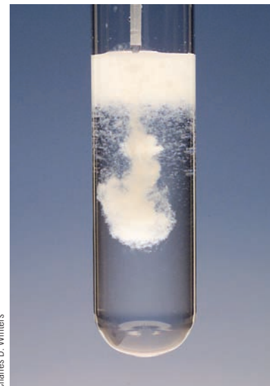
Figure 4.5 Precipitation of calcium carbonate ( \text{CaCO}_3 ). The precipitate forms when solutions of sodium carbonate ( \text{Na}_2\text{CO}_3 ) and calcium chloride ( \text{CaCl}_2 ) are mixed.
