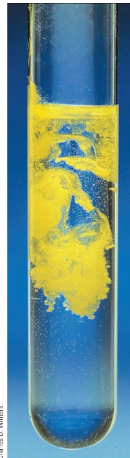
Figure 15.3 Precipitation of strontium chromate. A solution prepared by mixing solutions of \text{Sr}(\text{NO}_3)_2 and \text{K}_2\text{CrO}_4 is in equilibrium with yellow \text{SrCrO}_4(s) . In such a solution [\text{Sr}^{2+}] \times [\text{CrO}_4^{2-}] = 3.6 \times 10^{-5} .
