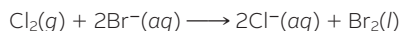
Figure 17.4 A \text{Cl}_2 - \text{Br}_2 voltaic cell. In this cell the spontaneous cell reaction is
