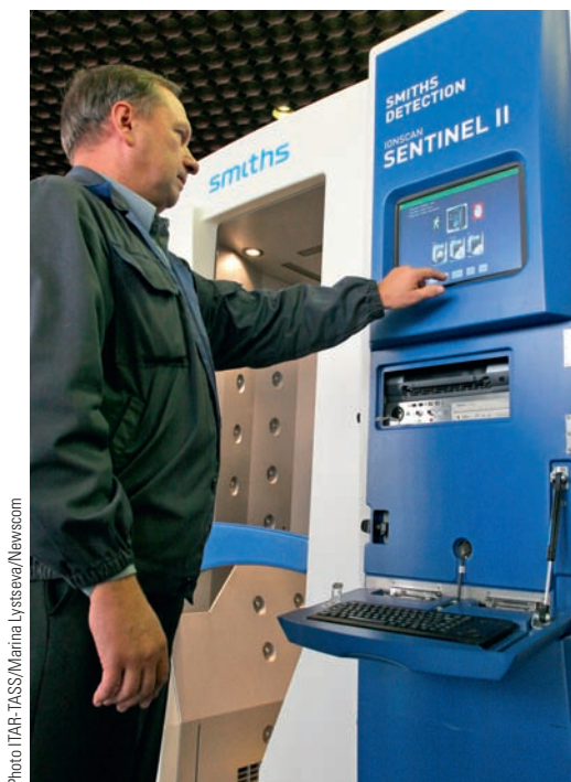
Figure 1.7 Chromatography and mass spectrometry applied to airport security. Airport security portals combine the separation of mixtures by chromatography with the detection of separated compounds such as explosives by mass spectrometry. A puff of air is used to collect a sample; even the smallest traces of such materials can be detected accurately and quickly. Larger versions of the same instrumentation can be used to scan checked baggage.
