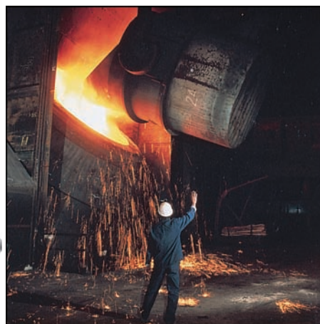
Figure 20.4 Iron and steel production. (a) A blast furnace for the production of pig iron. (b) A basic oxygen furnace, where the carbon content of pig iron is lowered by heating it with oxygen to form steel.
