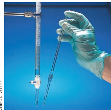
Figure 1.8 Measuring volume. A buret ( left ) delivers an accurately measured variable volume of liquid. A pipet ( right ) delivers a fixed volume (e.g., 25.00 mL) of liquid.
