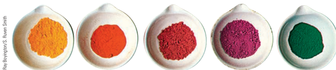
Figure 19.12 A spectrochemical series. The five cations listed in Table 19.3 vary in color from yellow [\text{Co}(\text{NH}_3)_6]\text{Cl}_3 to green [\text{trans-Co}(\text{NH}_3)_4\text{Cl}_2]\text{Cl} .
