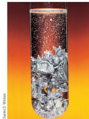
Figure 4.11 Redox reaction of zinc with a strong acid. The zinc atoms are oxidized to Zn 2+ ions in solution; the H + ions are reduced to H 2 molecules.
