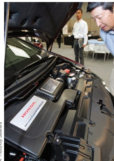
Fuel cell under Honda Clarity hood.
