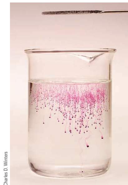
Figure 6.3 Crystals of potassium permanganate falling into water. The purple color of the solution results from absorption at approximately 550 nm.
