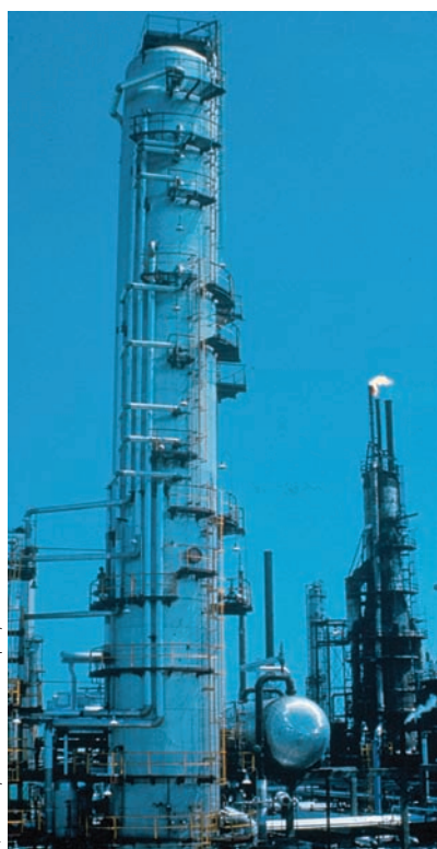
Figure 22.4 Petroleum distillation. (a) A distillation tower at a petroleum refinery. (b) A diagram showing the boiling points of the petroleum fractions separated by distillation.
