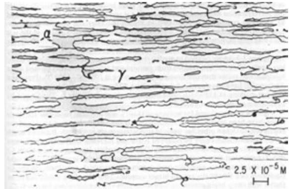
Figure 2 Typical duplex microstructure (reproduced by permission of ASM International from 'Duplex Stainless Steels,' 1983, pp. 693-756).
