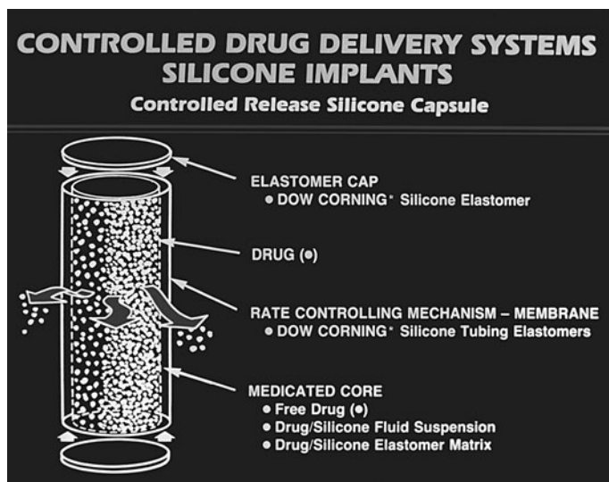
Figure 4.16 A controlled release drug-delivery system that utilizes both siloxane elastomers and fluids. The photograph was generously provided by the Dow Corning Corporation of Midland, MI.
