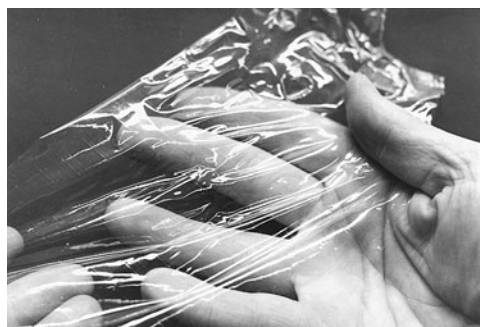
Figure 3.13 A thin film of poly[ bis (butyl-amino)phosphazene] fabricated by solution casting for membrane experiments.
