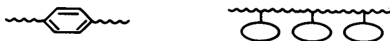
Figure 4.4 Some ways for making a polymer more rigid. 92 Reproduced by permission of John Wiley and Sons.
