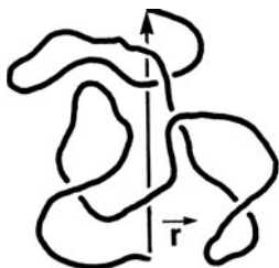
Figure 2.20 Representation of the end-to-end distance of a random-coil polymer. Reprinted with permission from J. E. Mark, “Physical Chemistry of Polymers,” ACS Audio Course C-89, American Chemical Society, Washington, DC, 1986. Copyright 1986, American Chemical Society.
