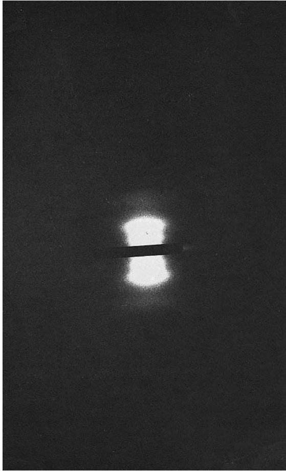
Fig. 1.8 Low-angle x-ray diffraction pattern of an axially oriented crystalline linear polyethylene specimen.(33)
