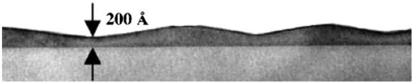
Figure 13.5. Cross-sectional TEM of a Si 0.8 Ge 0.2 /Si layer deposited at 630°C. From Phys. Rev. B 59 , 1990(1999) with permission. © 1999 American Physical Society.
