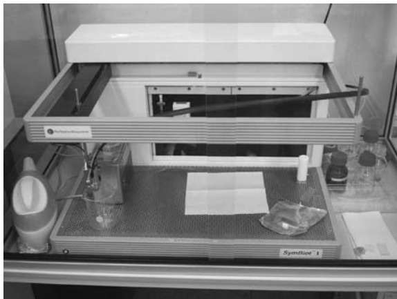
Fig. 2. Photograph of the in-house developed air driven spray station.
