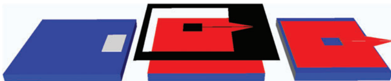
Figure 5.16 Novel fabrication process for the third generation of micromachined electrospray emitter tips: silicon support wafer (blue), 200 nm thick silicon dioxide etch-release layer (white) which is patterned using a HF-based wet-etch step, single polySi micro-nib layer (red) housing the reservoir and the nib tip which is defined using either a chlorine- or an SF 6 -based dry etch and single UV photolithographic masking step (black).
