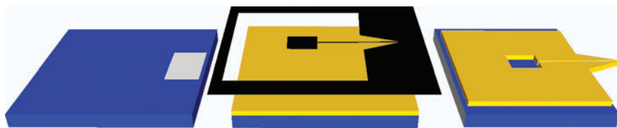
Figure 5.9 Novel fabrication process for the second generation of micromachined electro spray emitter tips: silicon support wafer (blue), 200 nm thick nickel etch-release layer (white) which is patterned using a HNO 3 -based wet etch, negative photoresist SU-8 which forms the micro-nib support layer and tip which hosts the capillary slot (gold) and single photolithographic masking layer which defines the reservoir and tip (black).
