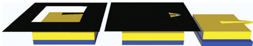
Figure 5.3 Novel fabrication process developed for manufacture of the first generation of micromachined electro spray emitter tips: silicon support wafer (blue), 400 \mu\text{m} thick negative photoresist SU-8 micro-nib layer (gold) and two-step UV photolithographic masking step (black) to form the reservoir structure and SU-8 support (using a long lithography exposure time) and the nib-like emitter tip containing the capillary slot (using a shorter lithography exposure time).
