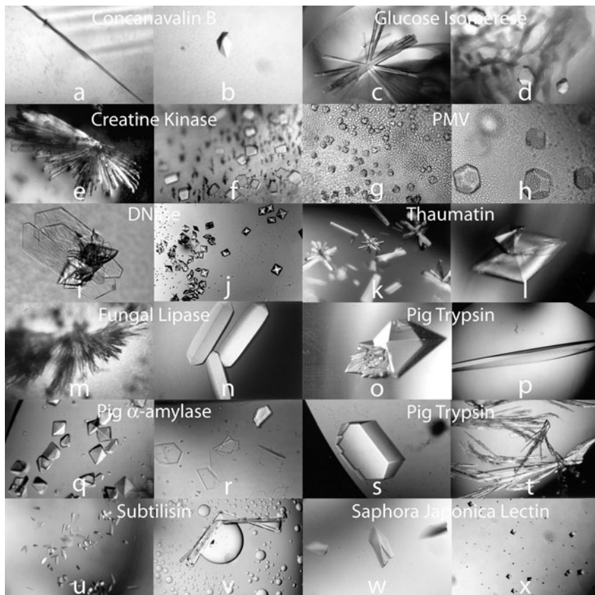
Figure 1.7. Gallery of pictures illustrating a variety of protein crystals. Note the wide variety of shapes. Note also the variation in the perfection of the external appearance of the crystals, which is not necessarily related to perfection in internal order. The names of the proteins appear in the individual frames. Kindly provided by Alexander McPherson.
