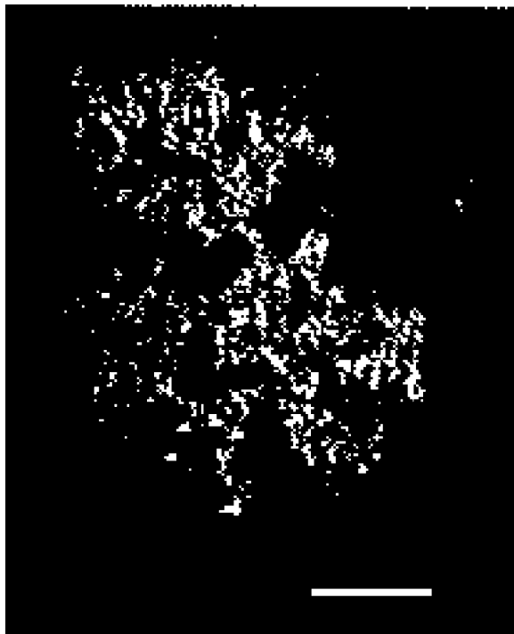
Figure 11.9 Brewster angle microscopy image taken at the Brewster angle of water at room temperature of a dipalmitoylphosphatidylethanolamine (DPPE) island on the air–water interface of an LB trough. Scale bar = 2 \mu\text{m} .
