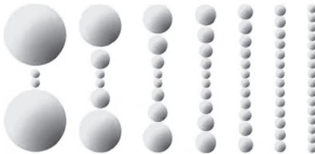
Figure 1.5 Gold nanosphere assemblies used in theoretical calculations by Chien et al. The length of each chain is fixed to equal 167.5 nm [16].
