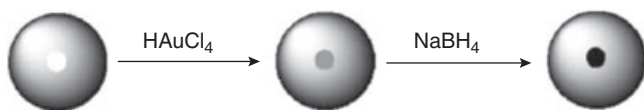
Scheme 10.3 Graphical representation of Au/SiO 2 formation via hollow silica nanoparticles. Reproduced with permission from Ref. [158]; © 2007, The Royal Society of Chemistry.
