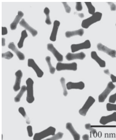
Figure 2.1 Transmission electron microscopy image of dumbbell-shaped Au/Ag nanoparticles. The contrast indicates the core-shell structure, with the bright segments indicating silver. Reprinted with permission from Ref. [4]; © 2004, American Chemical Society.
