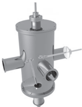
Figure 12.3 Simulated image of an arc-discharge chamber. The conductive ingots are mounted as both anodes and cathode (the end of yellow lines).
