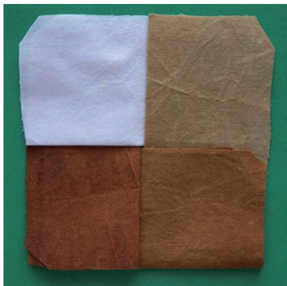
Figure 14.2 Cotton fabrics treated with increasing concentrations of silver nanoparticles. Before treatment the fabric is white; the color changes from light to dark brown with increasing silver concentrations.
