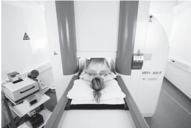
Figure 6.11 Thermotherapy treatment of the pelvic region after intratumoral injection of magnetic nanoparticles using the alternating magnetic field applicator MFH 300F® (MagForce Nanotechnologies AG, Berlin, Germany). Reprinted with permission from Ref. [175].
