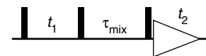
The pulse sequence for EXSY (and NOESY). All pulses have 90^\circ flip angles.
