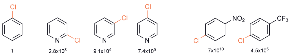
Rates of displacement of chloride by MeO - relative to chlorobenzene, at 50 °C
