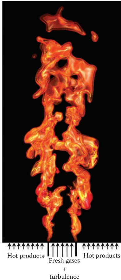
FIGURE 7.3.3 DNS of a slot-burner premixed flame. (From Sankaran, R. et al., Thirty-First International Symposium on Combustion , 2007.)
