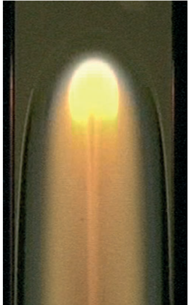
FIGURE 3.1.5 Schlieren picture of upward propagating rich limit propane flame with superimposed direct photography.
