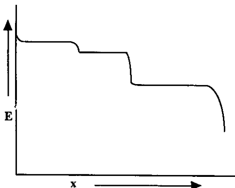
Fig. 10.6 Schematic equilibrium discharge curve of an electrode that undergoes a series of multi-phase reactions in which the residual value of F is zero
