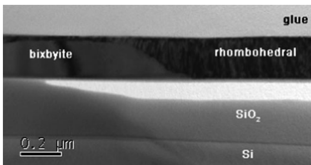
Fig. 4.13 Cross-sectional TEM image showing a crystallized IZO sample that contains both the bixbyite and the rhombohedral phase of IZO
