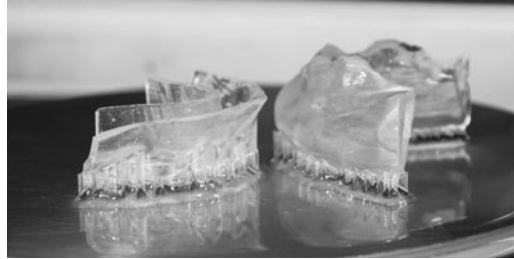
Fig. 7.11 A 3D model of the upper dental arch produced by stereolithography. Drilling guide for inserting dental implants. Courtesy of Materialise Dental (F. Maes)
