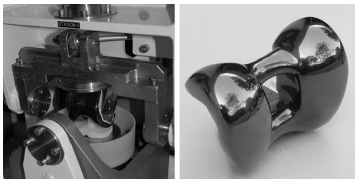
Fig. 5.5 In vitro 4-axis testing machine for prostheses. The device simulates the in vivo behavior: on the picture a total knee prosthesis under test. Courtesy Smith & Nephew
