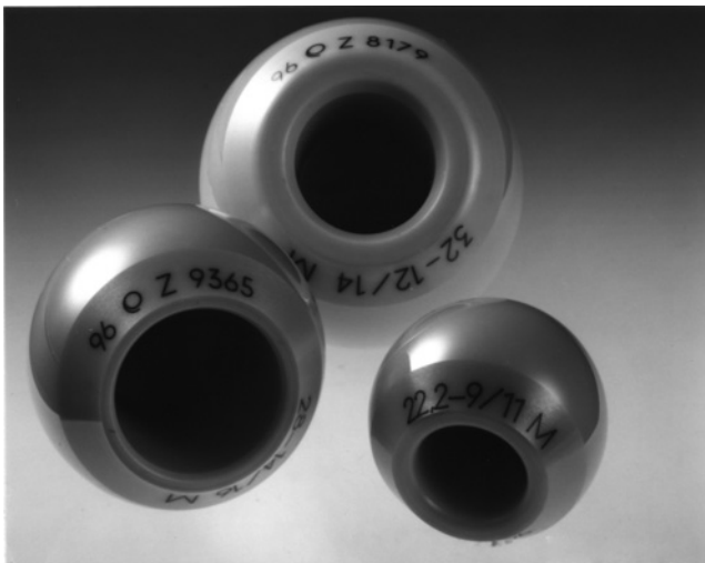
Figure 10.30 Laser markings of zirconia femoral ball heads (Heimann and Willmann, 1998). For details, see the text.
