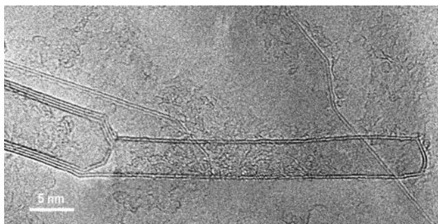
Fig. 2.8 Nanotube structure found in a commercial graphite.
