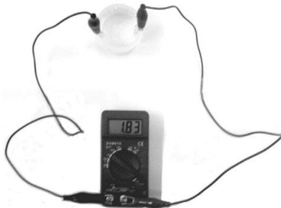
Figure 5-8 The platinum fuel cell generating electricity.
