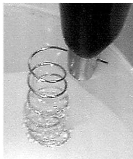
Figure 5-4 Close-up of the wires clipped snugly to the inside of the container.
