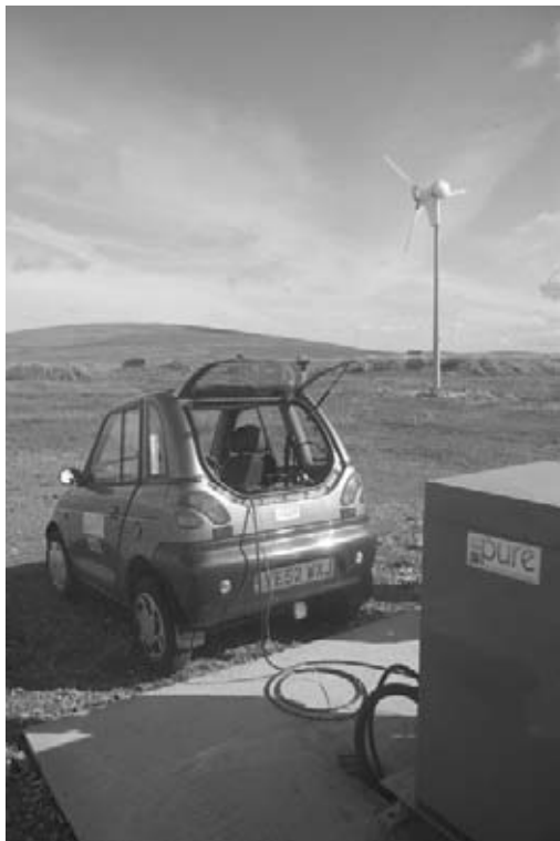
Figure 4-23 PURE Energy Centre fuel cell car fitted with metal hydride hydrogen storage.
