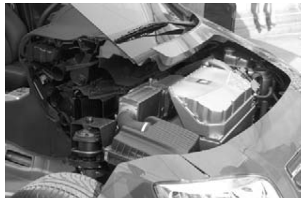
Figure 13-4 Under the hood of a fuel cell car.
