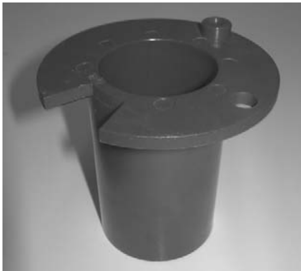
Figure 6-9 The mini alkaline fuel cell cathode assembly.
