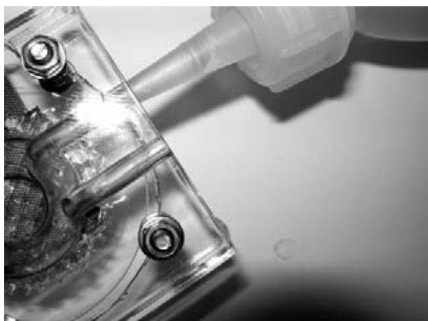
Figure 8-5 Closeup of filling the methanol fuel cell.
