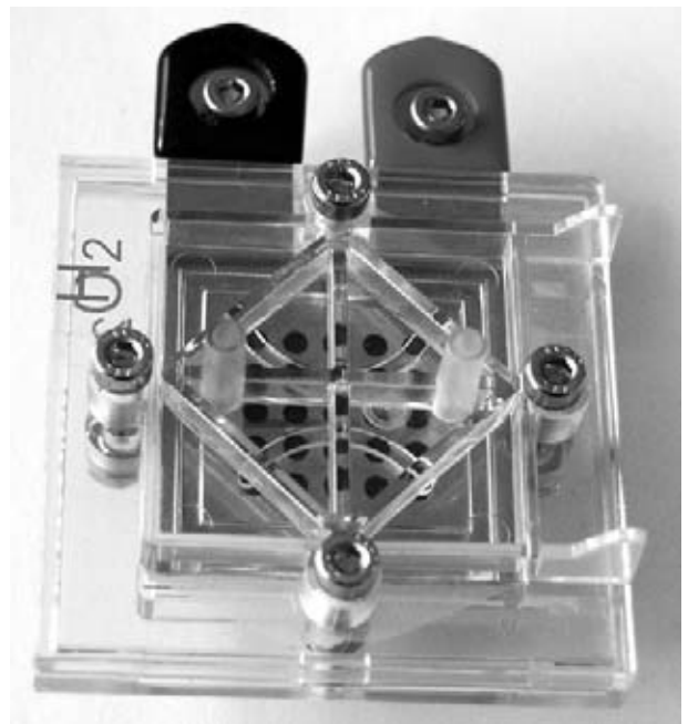
Figure 7-14 The complete dismantlable fuel cell.
