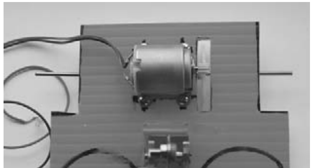
Figure 13-27 Axle and large gear wheel installed.
