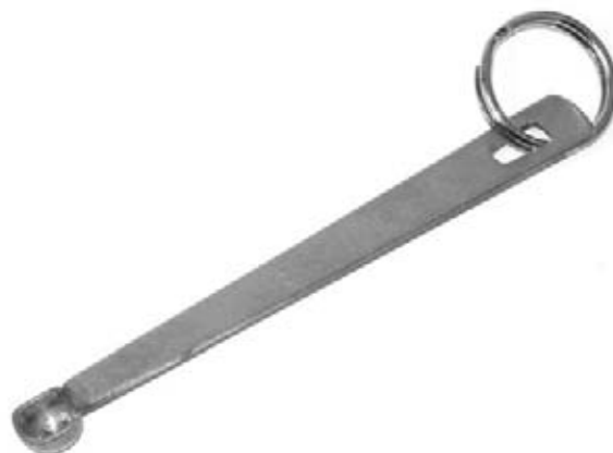
Figure 4-17 Spatula used to measure the quantity of sodium borohydride.
