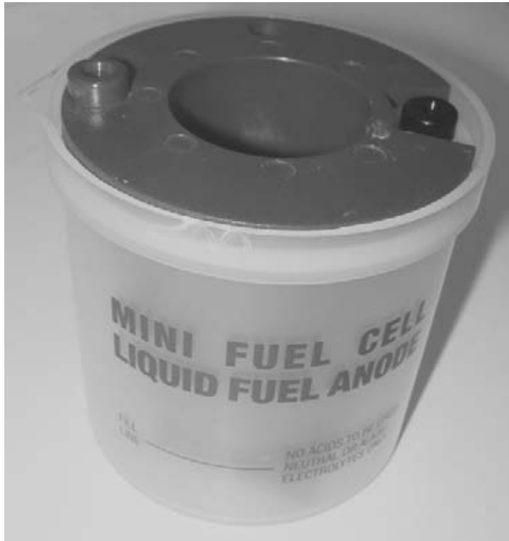
Figure 6-6 The assembled mini alkaline fuel cell.
