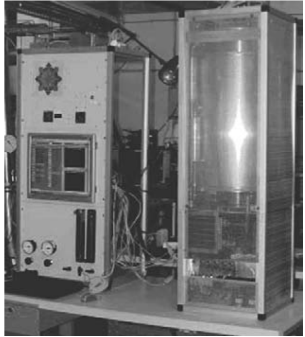
Figure 10-2 Solid oxide fuel cell stack and support equipment in the lab. Image courtesy Technology Management Inc.
