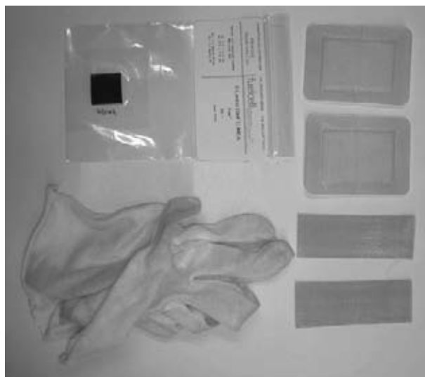
Figure 8-7 The components of the Band-Aid fuel cell.
