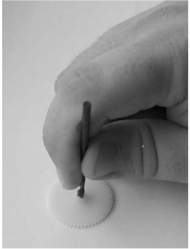
Figure 13-26 Use a small drill to enlarge the axle hole.
