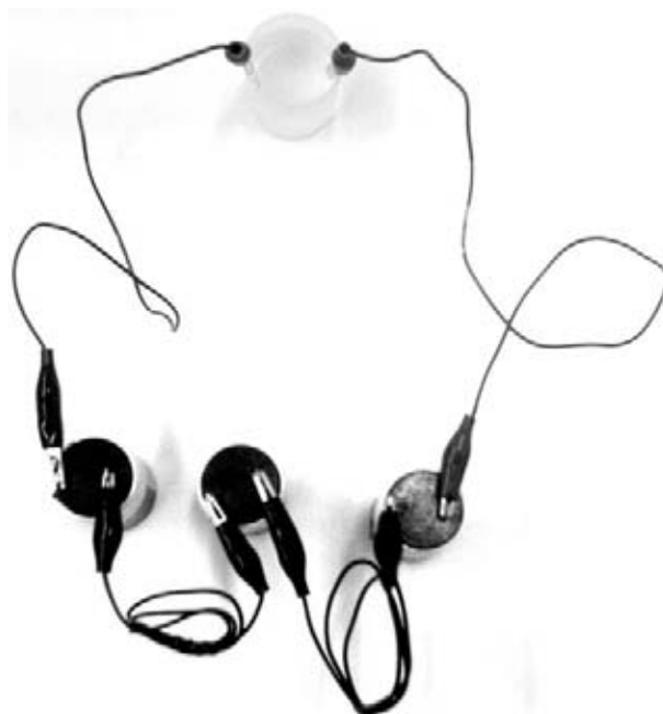
Figure 5-6 A picture of the completed setup for electrolysis.
