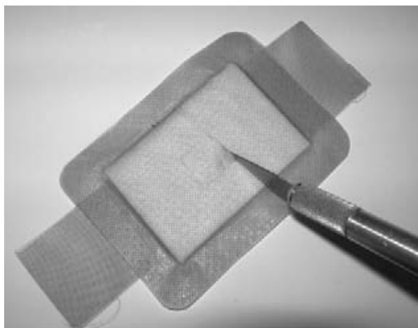
Figure 8-20 Using a scalpel to remove a square from the top layer of the Band-Aid (initial cut).
