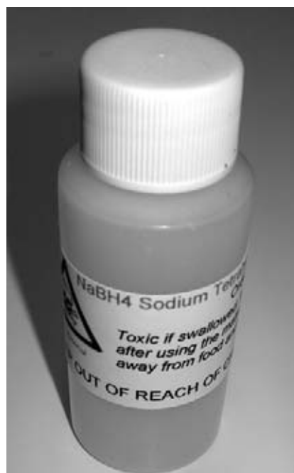
Figure 6-12 Sodium borohydride, the source of hydrogen for our AFC.
