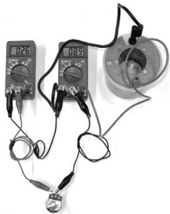
Figure 6-18 The alkaline fuel cell measurement setup.
