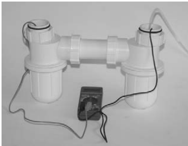
Figure 9-4 The completed microbial fuel cell.
