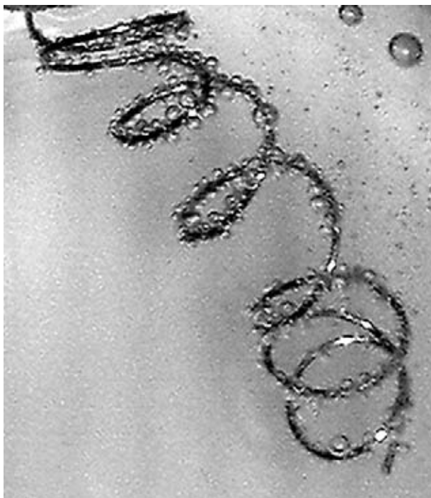
Figure 5-9b Close-up of the hydrogen electrode.
