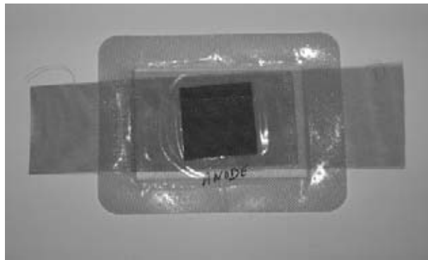
Figure 8-19 Laying the final layer of wire mesh on top of the MEA.
