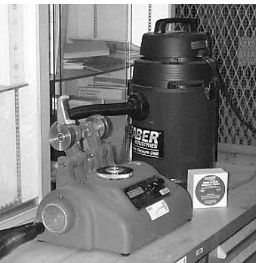
Figure 13.5 Taber abrasion apparatus. (Courtesy of Martin Testing Laboratories, Inc.)
