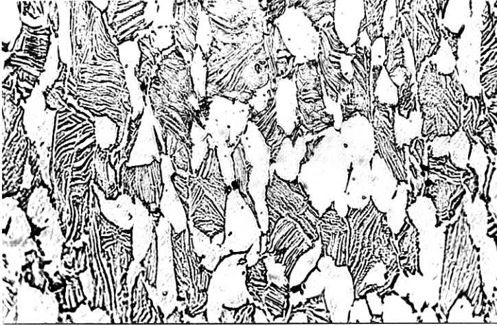
Figure 3.3 Equiaxed \alpha plus lamellar transformed \beta grains (Ti-6-4, 960°C, air cool).
