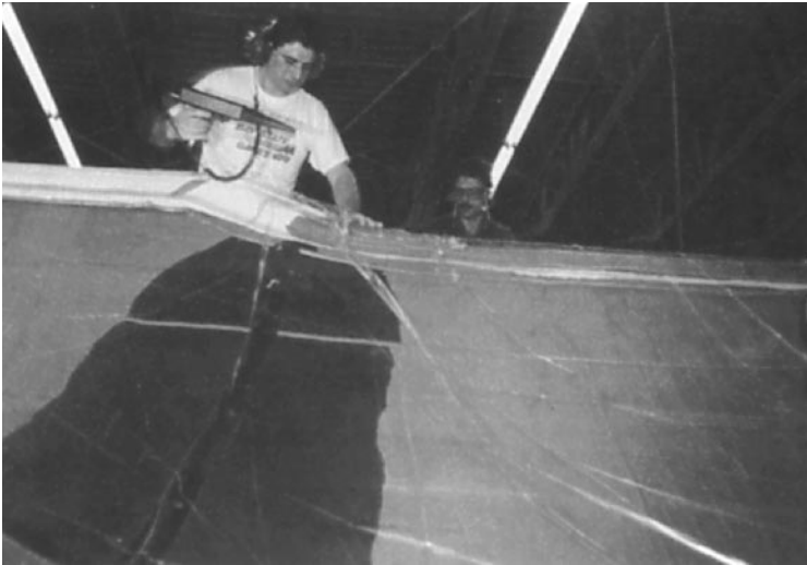
Figure 5.17 RTM (SCRIMP™) process for injecting a boat hull. (Copyright Billy Black, courtesy of Seemann Composites)
