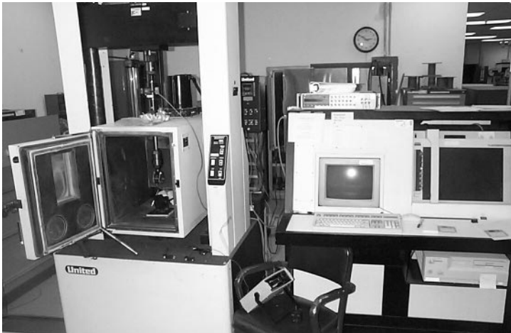
Figure 13.4 Automated tensile testing equipment with a thermal chamber for hot/cold testing of materials. Source: Courtesy of Martin Testing Laboratories, Inc.
