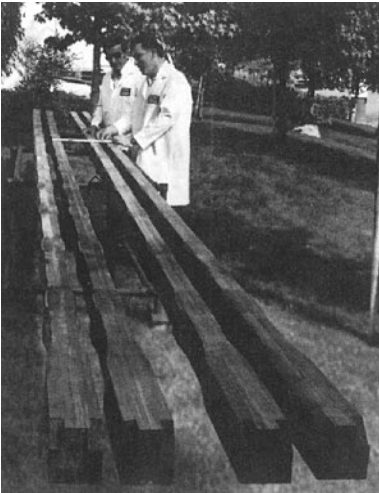
Figure 5.24 Filament-wound/protruded graphite epoxy bridge beam. (Courtesy of Sci. Div. of Harsco.)
