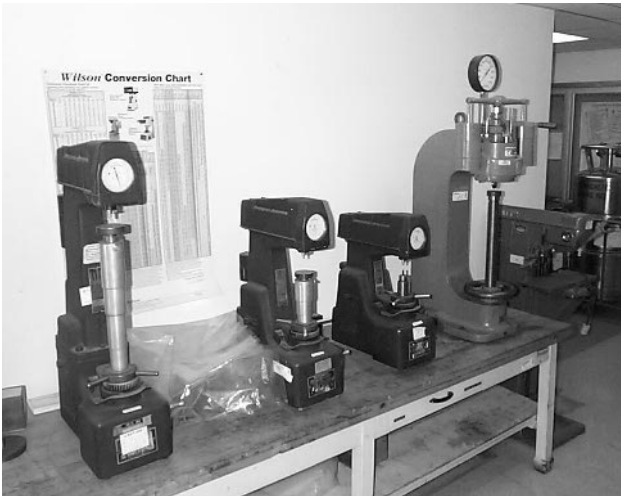
Figure 13.3 From left to right, Rockwell C tester, Rockwell B tester, Superficial Rockwell tester, and Vickers tester (on floor). (Courtesy of Martin Testing Laboratories.)
