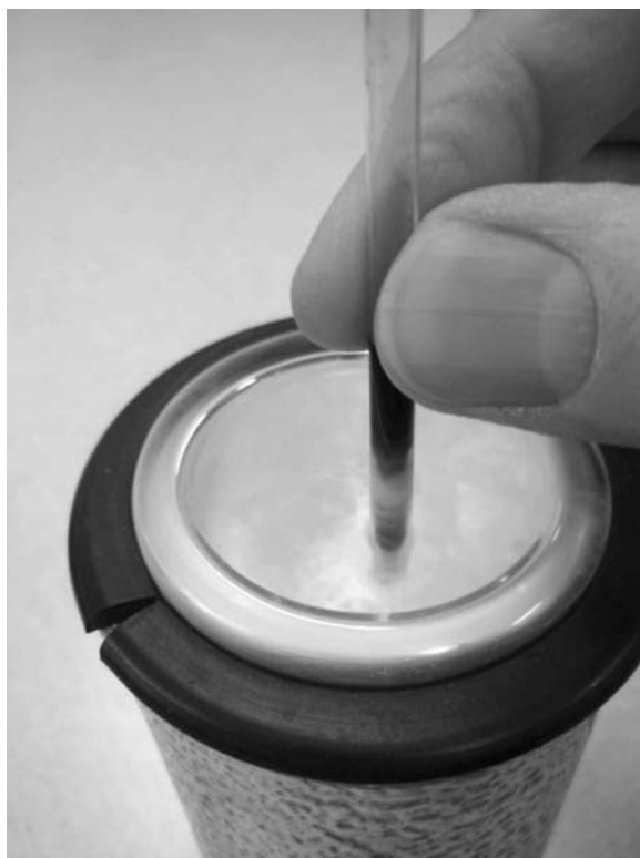
FIGURE 3.3 Fail-safe recipe for freezing EPR samples. The tube is held just above the sample, which is allowed to freeze and expand from the bottom to the top.
