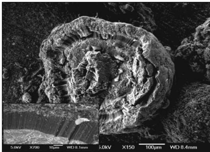
Figure 11.3 SEM images of aligned CNTs prepared by CVD on spherical supports.
