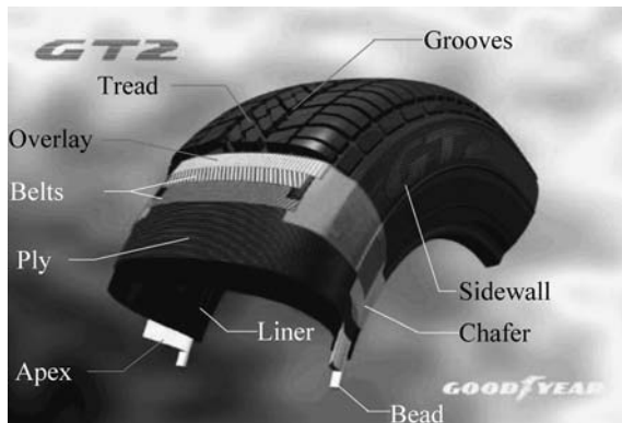
Figure 8.5 Schematic of a pneumatic radial tire.
