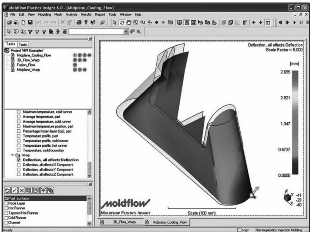
Figure 4.51 Simulation of injection molding showing the many drop-down menus of the MOLDFLOW software [44].
