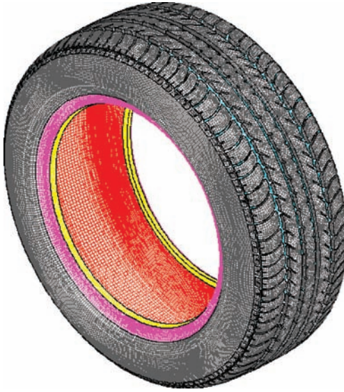
Figure 8.9 Treaded tire model.
