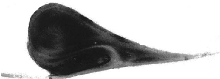
Figure 4.23 Experimental flow pattern in the melt bank of calendered rigid PVC [78, 79].
