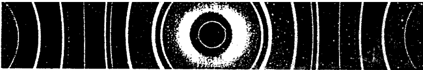
Figure 2.27. Film recorded in a Debye-Scherer and Hull diffractometer with a sample of zinc oxide
