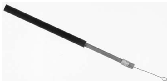
Figure 3.3 A nichrome loop for the inoculation of solid and liquid media with organisms
