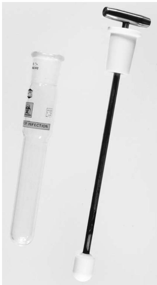
Figure 4.19 A tissue homogenizer for preparing fungal inocula
