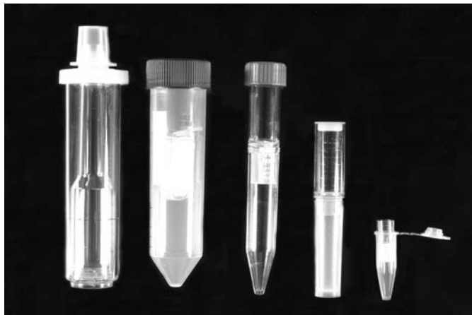
Figure 6.10 A range of membrane concentrator units for concentration of protein solutions in centrifuges
