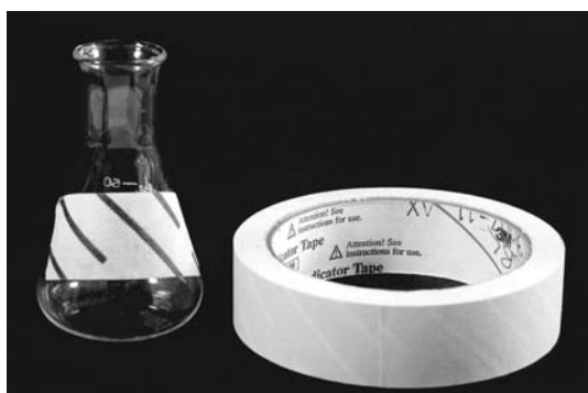
Figure 3.9 Autoclave tape, showing black stripes that develop on heating
