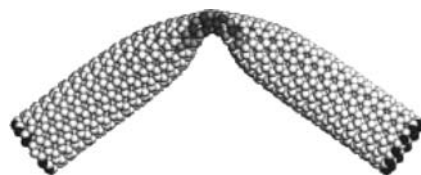
FIGURE 4.9 MD simulation of a large-amplitude transverse deformation of a carbon nanotube, apparently beyond the elastic limit. In fact, the tube snaps back once the computer-generated force is removed, and there is no plastic deformation or permanent damage. (From Yakobson, B. I., Appl. Phys. Lett. 72 , 918–920 (1998), with permission.)
