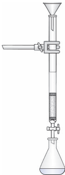
Figure 6.11 Set-up for column chromatography.
