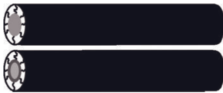
Figure 2.1 Structural illustration of a diblock nanofiber (top) and a triblock nanofiber (bottom).
