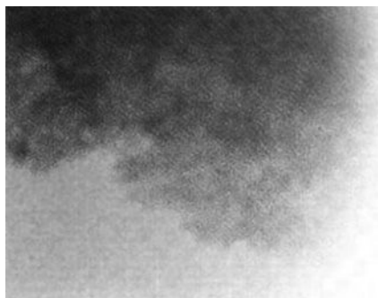
Figure 15.4 Transmission electron microscopy image of the MSU-1 alumina prepared with a surfactant of Tergitol® 15-S-9 and calcined at 500 °C. Scale bar = 60 nm. Reprinted with permission from Ref. [5a].
