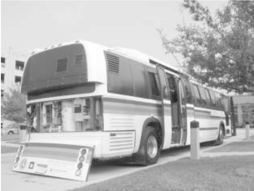
6.10 The 'Georgetown Bus.' A 100kW PAFC powered bus that is fueled by methanol.
