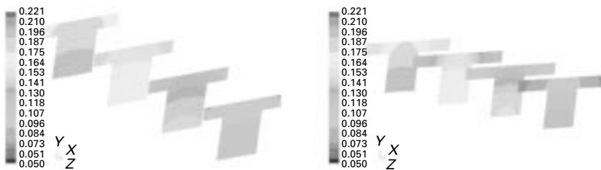
4.28 Oxygen concentration profile (50% utilization) at a single channel/rib system at a current density of 0.4 \text{ A/cm}^2 (1 and 2 mm rib width, 1 mm channel depth).
