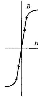
Figure 6.49 Hysteresis loop for a magnetically soft material. In the ideal case the enclosed area of the loop is zero. Reproduced with permission from A. G. Guy, Elements of Physical Metallurgy , 2nd edn. © Addison-Wesley Publishing Company, Inc. (now under Pearson Education).
