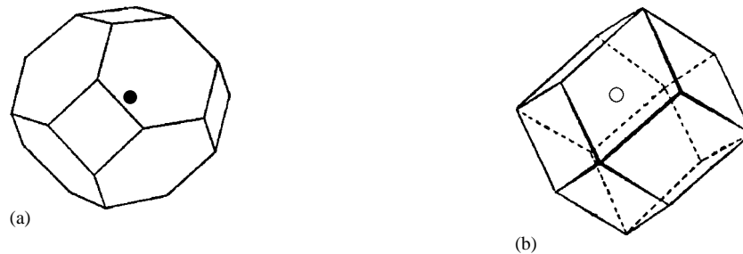
Figure 3.45 (a) Primitive unit cell (Wigner–Seitz cell) of a BCC crystal. • = origin in r space. (b) The first Brillouin zone (Wigner–Seitz cell in k space) of a BCC crystal is an FCC polyhedron. ◦ = origin in k -space. Reproduced with permission from W. Hume-Rothery and B. R. Coles, Atomic Theory for Students of Metallurgy . (Published by the Institute of Metals, 1969.) now © W. S. Maney & Son Ltd.
