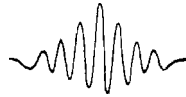
Figure 2.5 A quantum h\nu is regarded as a small group of waves which amplify each other by constructive interference within a limited region and destroy each other by destructive interference elsewhere in space.
