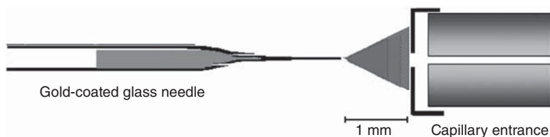
Figure 1.10. Typical instrumental configuration for nano-ESI experiments.
