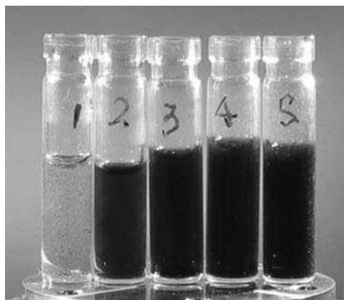
Figure 19.19 Pictures of five nanofiller (nanotube) solutions with different functional groups and chemical structures. (Reproduced with kind permission from NLGI. Copyright (2010) NLGI)
