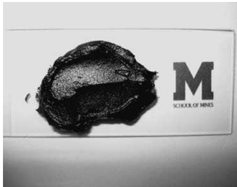
Figure 19.7 Picture of the nanocomposite (grease) made from the nanofiller (carbon nanotubes) and polymer (DURASYN® 166 oil). (Reproduced with kind permission from NLGI. Copyright (2010) NLGI)
