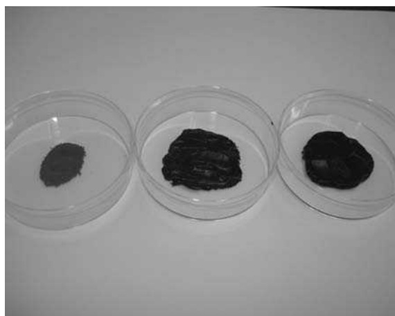
Figure 19.14 Picture of several materials: (A) \text{Fe}_2\text{O}_3 nanoparticles; (B) grease made from 10 wt% SWNTs and 10 wt% \text{Fe}_2\text{O}_3 ; and (C) grease made from 10 wt% SWNTs. (Reproduced with kind permission from NLGI. Copyright (2010) NLGI)
