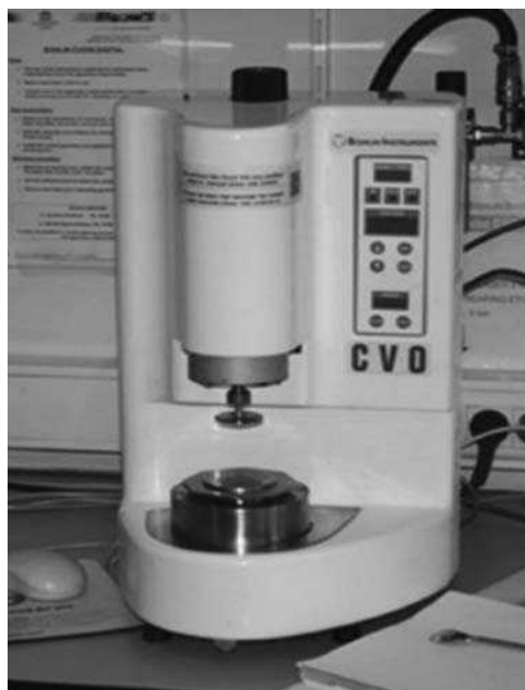
Figure 19.6 Bohlin CVO-controlled stress rheometer. (Reproduced with kind permission from NLGI. Copyright (2010) NLGI)
