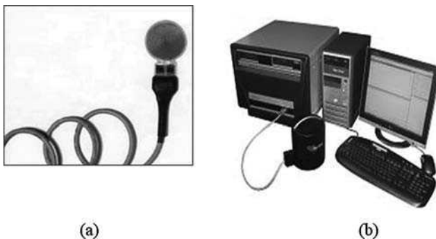
Figure 19.3 Hot Disk™ thermal constants analyzer: (a) sensor; (b) equipment diagram. (Reproduced with kind permission from NLGI. Copyright (2010) NLGI)
