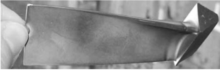
Figure 1.30 A small helicopter turbine blade covered by magnetron plasma sputtering with a 0.3-mm thick Al-Co-Fe-Cr thermal barrier. The thumbnail on the left gives an approximate scale for the figure (Courtesy S. Drawin, Onera, France).
