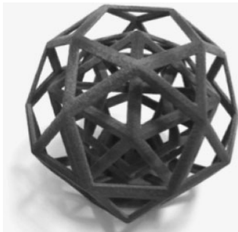
Figure 1.31 Example of a complex shape produced by laser selective rapid prototyping and sintering of a very complex shape of embedded polyhedra made of CMA powder in a polymer matrix. The object is a few cm in diameter.
