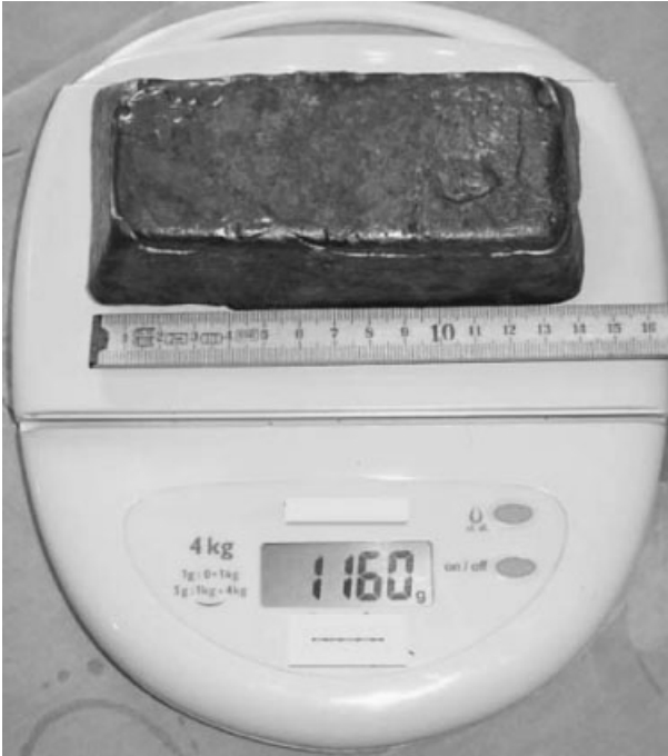
Figure 1.26 One of the many 1-kg ingots of \text{Al}_{62}\text{Cu}_{18}\text{Fe}_{10}\text{Cr}_{10} (at.%) CMA alloy that was prepared by a conventional metallurgical route for feeding a powder atomization tower and
