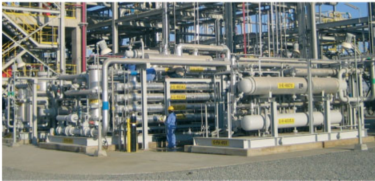
Figure 8.14 Flow diagram showing the use of hydrocarbon-permeable membranes to recover unreacted monomers from a polyolefin plant resin degassing unit. The photograph is of a system installed by MTR in Qatar in 2007.
