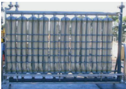
D: HF/CT membranes mounted in frame
