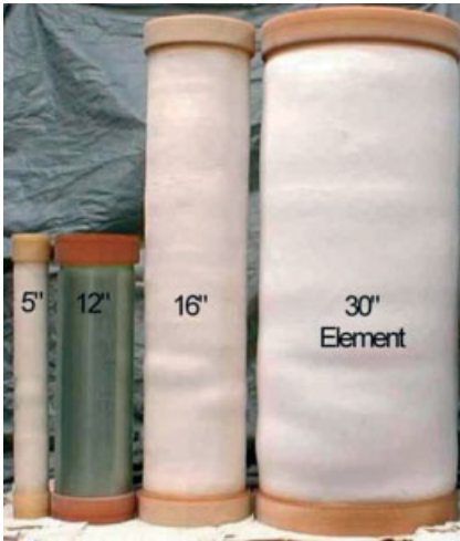
Figure 8.2 The expanding diameter of Cynara hollow-fiber membrane modules, from the first 5-inch modules of the 1980s to the 30-inch diameter behemoths now being introduced (Photo used courtesy of NATCO Group, Inc.) [9].
