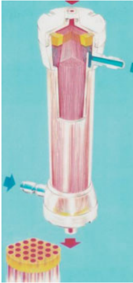
Figure 18.5 Cut out of a hollow-fiber dialyzer.
