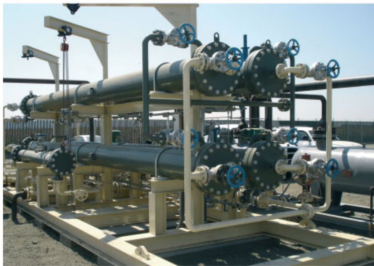
Figure 8.13 Flow diagram and photograph of a 12 MMscfd membrane nitrogen removal plant installed on a high-nitrogen gas well in the Sacramento River Delta region of California. Reproduced with permission from Ind. Eng. Chem. Res. 2008, 47 (7), 2109–2121. Copyright 2008 American Chemical Society [17].
