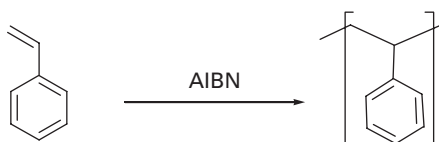
Scheme 5 Polymerization of styrene initiated by AIBN.
