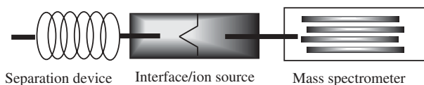
Figure 5.1. Conceptual diagram of the coupling of a separation device with a mass spectrometer.
