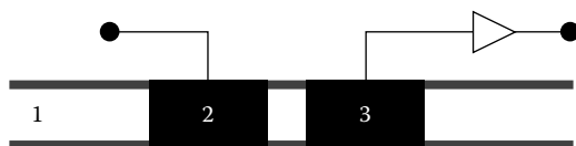
FIGURE 6.5 Schematic representation of contactless conductivity detection cell. (1) Capillary, (2) actuator electrode, and (3) pickup electrode.
