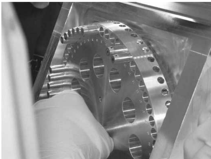
Figure 16.4 View of the wheel holding several samples to be measured. The photograph is from the HVEE 846b source at the LABEC laboratory in Florence
