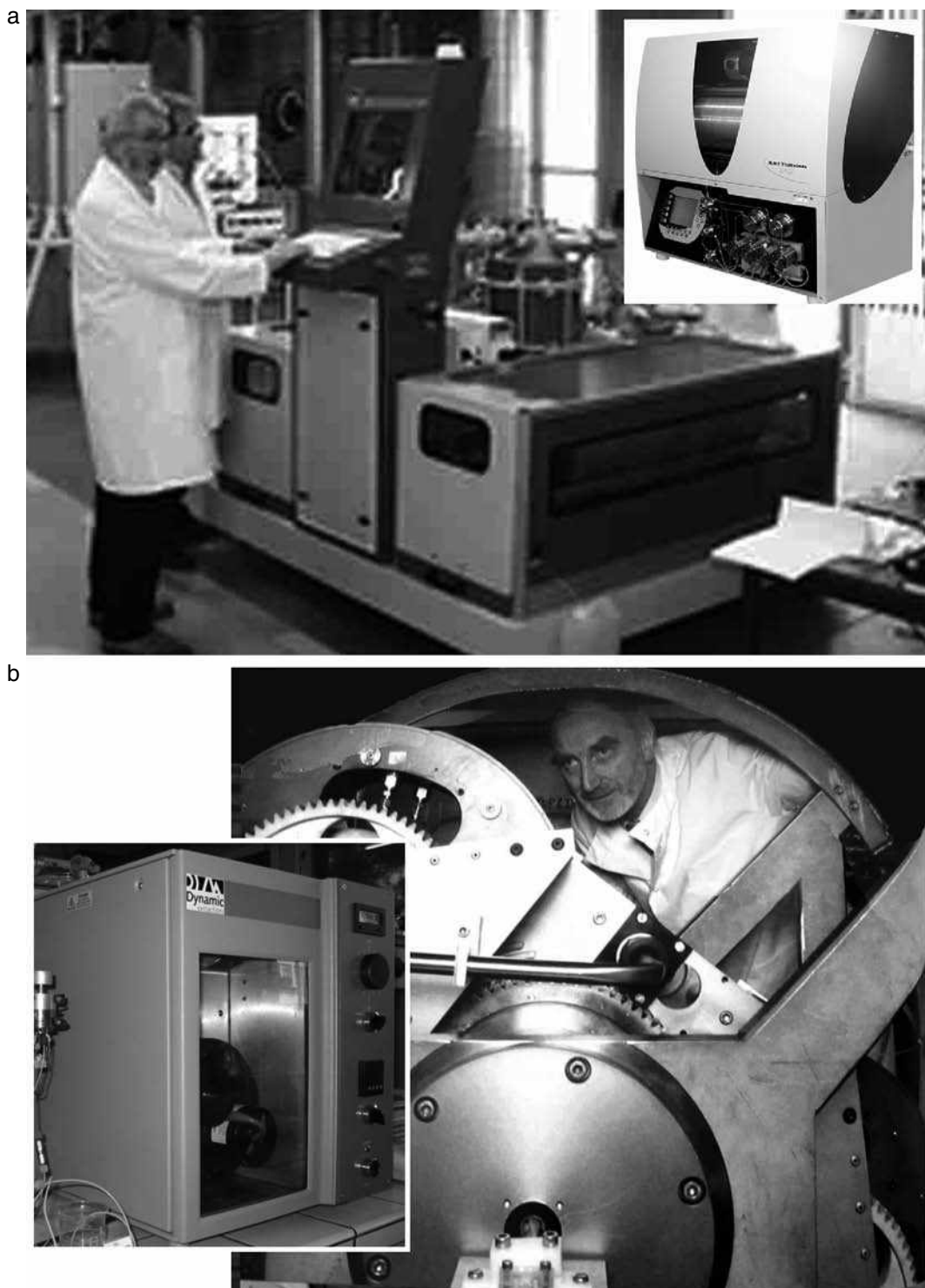
Fig. 1 Countercurrent chromatography columns. a, The hydrostatic Armen Elite CPC12L with two 6 L rotors. The inset shows the small Elite CPC250 (0.25 L column) ( http://www.armen-instrument.com and Table 1); b, The hydrodynamic Maxi 5 L column. Pr. Ian Sutherland (Brunel University, Uxbridge, U.K.) poses inside the rotor to give the scale. The inset shows the Spectrum 20 ml column ( http://www.dynamicextractions.com and Table 1).
