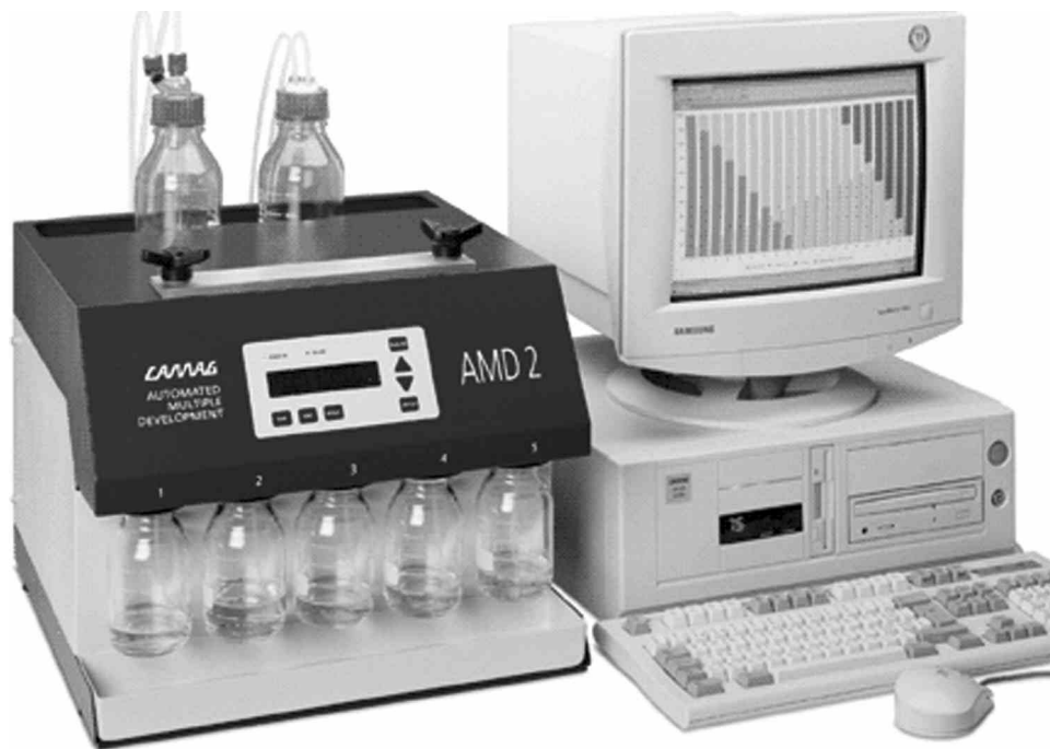
Fig. 5 Device for automated multiple development (AMD2). Source: Courtesy of Camag. [5]
