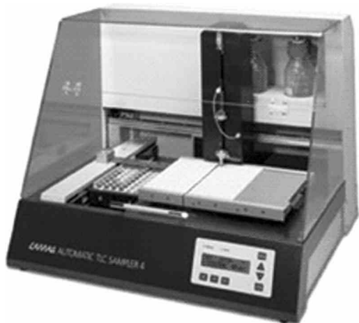
Fig. 4 Full automatic applicator (ATS 4). Source: Courtesy of Camag. [5]
