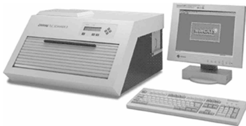
Fig. 7 Densitometer linked with personal computer. Source: Courtesy of Camag. [5]
