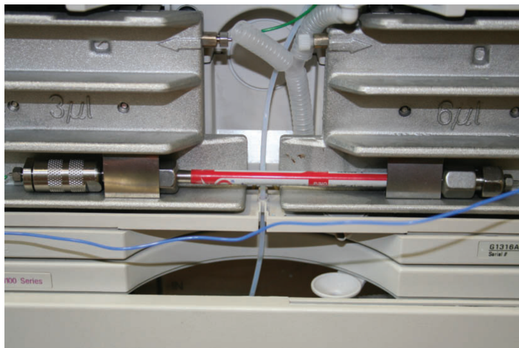
Plate 14 HPLC column in the opened column chamber (photo: G. Merkh, University of Hohenheim).
