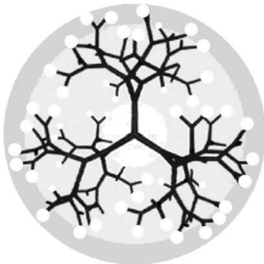
FIGURE 13.1 A dendrimer with its branching units, its core, and its internal voids. Modified image taken from: http://www.nisenet.org/image/dendrimer (unknown author)
