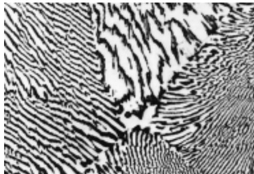
FIGURE 10.12 Photomicrograph showing the microstructure of a lead–tin alloy of eutectic composition. This microstructure consists of alternating layers of a lead-rich \alpha -phase solid solution (dark layers), and a tin-rich \beta -phase solid solution (light layers). 375 \times . (Reproduced with permission from Metals Handbook , Vol. 9, 9th edition, Metallography and Microstructures , American Society for Metals, Materials Park, OH, 1985.)
