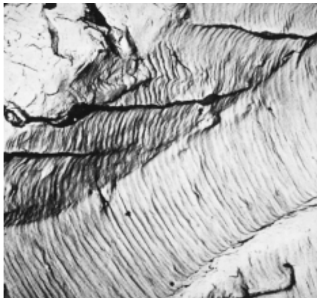
FIGURE 9.31 Transmission electron fractograph showing fatigue striations in aluminum. Magnification unknown. (From V. J. Colangelo and F. A. Heiser, Analysis of Metallurgical Failures , 2nd edition. Copyright © 1987 by John Wiley & Sons, New York. Reprinted by permission of John Wiley & Sons, Inc.)
