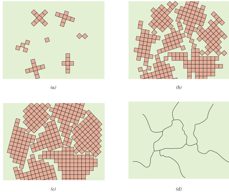
Figure 3.18 Schematic diagrams of the various stages in the solidification of a polycrystalline material; the square grids depict unit cells. (a) Small crystallite nuclei. (b) Growth of the crystallites; the obstruction of some grains that are adjacent to one another is also shown. (c) Upon completion of solidification, grains having irregular shapes have formed. (d) The grain structure as it would appear under the microscope; dark lines are the grain boundaries. (Adapted from W. Rosenhain, An Introduction to the Study of Physical Metallurgy , 2nd edition, Constable & Company Ltd., London, 1915.)
