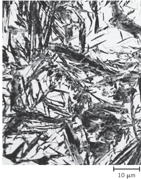
Figure 10.21 Photomicrograph showing the martensitic microstructure. The needle-shaped grains are the martensite phase, and the white regions are austenite that failed to transform during the rapid quench. 1220 \times . (Photomicrograph courtesy of United States Steel Corporation.)
