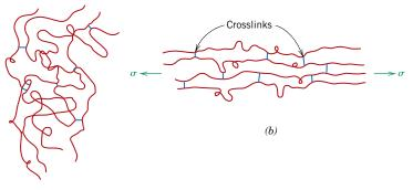
the chains spring back to their prestressed conformations, and the macroscopic piece returns to its original shape.
