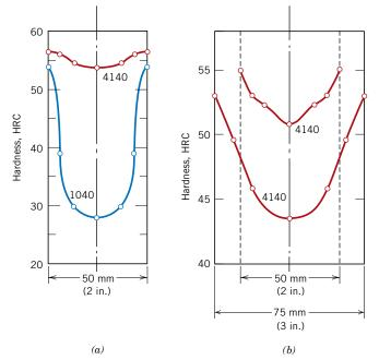
Figure 11.18 Radial hardness profiles for (a) 50 mm (2 in.) diameter cylindrical 1040 and 4140 steel specimens quenched in mildly agitated water, and (b) 50 and 75 mm (2 and 3 in.) diameter cylindrical specimens of 4140 steel quenched in mildly agitated oil.
