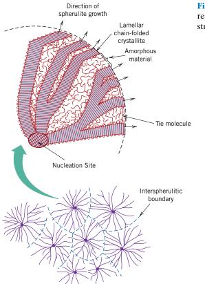
**Figure 14.13** Schematic representation of the detailed structure of a spherulite.
