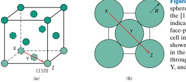
**Figure 3.12** (*a*) Reducedsphere FCC unit cell with the [110] direction indicated. (*b*) The bottom face-plane of the FCC unit cell in (*a*) on which is shown the atomic spacing in the [110] direction, through atoms labeled X, Y, and Z.
