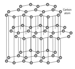
Figure 12.17 The structure of graphite.
