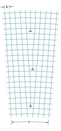
**Figure 4.8** Demonstration of how a tilt boundary having an angle of misorientation  $\theta$  results from an alignment of edge dislocations.
