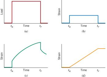
Elastic deformation is instantaneous, which means that total deformation (or strain) occurs the instant the stress is applied or released (i.e., the strain is independent of time). In addition, upon release of the external stress, the deformation is totally recovered—the specimen assumes its original dimensions. This behavior is represented in Figure 15.5*b* as strain versus time for the instantaneous load–time curve, shown in Figure 15.5*a*.
