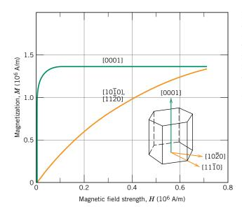
Figure 20.18 Magnetization curves for single crystals of cobalt. The curves were generated when the magnetic field was applied in [0001] and [1010]/[1120] crystallographic directions. [Adapted from S. Kaya, "On the Magnetisation of Single Crystals of Cobalt," *Sci. Rep. Tohoku Univ.*, **17**, 1157 (1928).]
