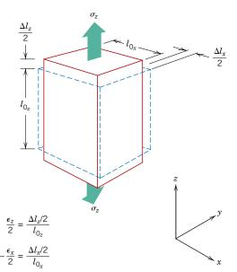
**Figure 6.9** Axial (z) elongation (positive strain) and lateral (x and y)contractions (negative strains) in response to an imposed tensile stress. Solid lines represent dimensions after stress application; dashed lines, before.
