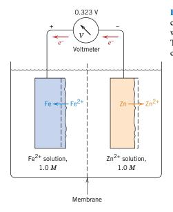
Figure 17.3 An electrochemical cell consisting of iron and zinc electrodes, each of which is immersed in a 1M solution of its ion. The iron electrodeposits while the zinc corrodes.
