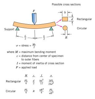
**Figure 12.32** A three-point loading scheme for measuring the stress–strain behavior and flexural strength of brittle ceramics, including expressions for computing stress for rectangular and circular cross sections.
