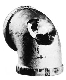
**Figure 17.20** Impingement failure of an elbow that was part of a steam condensate line. (Photograph courtesy of Mars G. Fontana. From M. G. Fontana, *Corrosion Engineering*, 3rd edition. Copyright © 1986 by McGraw-Hill Book Company. Reproduced with permission.)
