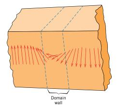
**Figure 20.12** The gradual change in magnetic dipole orientation across a domain wall. (From W. D. Kingery, H. K. Bowen, and D. R. Uhlmann, *Introduction to Ceramics*, 2nd edition. Copyright © 1976 by John Wiley & Sons, New York. Reprinted by permission of John Wiley & Sons, Inc.)
