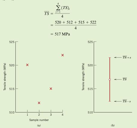
**Figure 6.20** (*a*) Tensile strength data associated with Example Problem 6.6. (*b*) The manner in which these data could be plotted. The data point corresponds to the average value of the tensile strength ( $\overline{TS}$ ); error bars that indicate the degree of scatter correspond to the average value plus and minus the standard deviation ( $\overline{TS} \pm s$ ).
