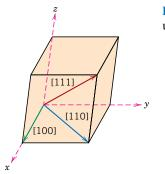
Figure 3.6 The [100], [110], and [111] directions within a unit cell.
