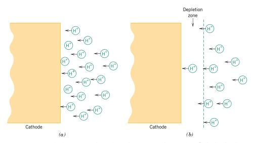
**Figure 17.8** For hydrogen reduction, schematic representations of the  $H^+$  distribution in the vicinity of the cathode for (*a*) low reaction rates and/or high concentrations, and (*b*) high reaction rates and/or low concentrations wherein a depletion zone is formed that gives rise to concentration polarization. (Adapted from M. G. Fontana, *Corrosion Engineering*, 3rd edition. Copyright © 1986 by McGraw-Hill Book Company. Reproduced with permission.)
