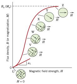
**Figure 20.13** The *B*-versus-*H* behavior for a ferromagnetic or ferrimagnetic material that was initially unmagnetized. Domain configurations during several stages of magnetization are represented. Saturation flux density  $B_s$ , magnetization  $M_s$ , and initial permeability  $\mu_i$  are also indicated. (Adapted from O. H. Wyatt and D. Dew-Hughes, *Metals, Ceramics and Polymers*, Cambridge University Press, 1974.)
