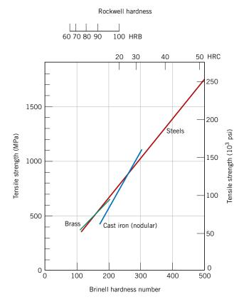
Figure 6.19 Relationships between hardness and tensile strength for steel, brass, and cast iron. [Data taken from Metals Handbook: Properties and Selection: Irons and Steels, Vol. 1, 9th edition, B. Bardes (Editor), American Society for Metals, 1978, pp. 36 and 461; and Metals Handbook: Properties and Selection: Nonferrous Alloys and Pure Metals, Vol. 2, 9th edition, H. Baker (Managing Editor), American Society for Metals, 1979, p. 327.]
