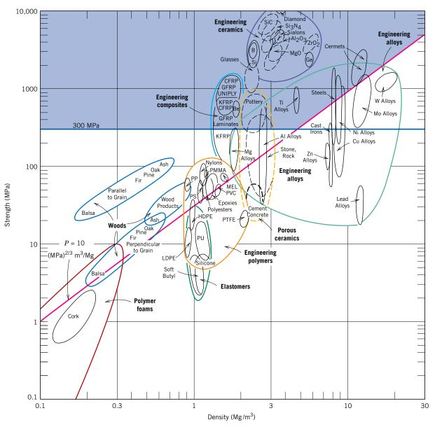
**Figure 22.3** Strength versus density materials selection chart. Those materials lying within the shaded region are acceptable candidates for a solid cylindrical shaft that has a mass-strength performance index in excess of 10 (MPa)<sup>2/3</sup>m<sup>3</sup>/Mg, and a strength of at least 300 MPa (43,500 psi). (Adapted from M. F. Ashby, *Materials Selection in Mechanical Design*. Copyright © 1992. Reprinted by permission of Butterworth-Heinemann Ltd.)
