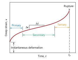
**Figure 8.28** Typical creep curve of strain versus time at constant stress and constant elevated temperature. The minimum creep rate  $\Delta \epsilon / \Delta t$  is the slope of the linear segment in the secondary region. Rupture lifetime  $t_r$  is the total time to rupture.
