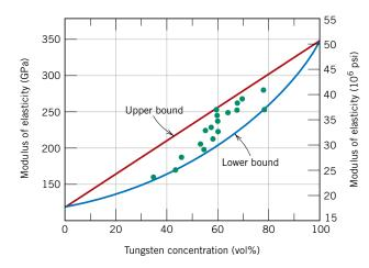
**Figure 16.3** Modulus of elasticity versus volume percent tungsten for a composite of tungsten particles dispersed within a copper matrix. Upper and lower bounds are according to Equations 16.1 and 16.2; experimental data points are included. (From R. H. Krock, *ASTM Proceedings*, Vol. 63, 1963. Copyright ASTM, 1916 Race Street, Philadelphia, PA 19103. Reprinted with permission.)
