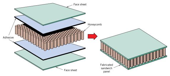
**Figure 16.18** Schematic diagram showing the construction of a honeycomb core sandwich panel. (Reprinted with permission from *Engineered Materials Handbook*, Vol. 1, *Composites*, ASM International, Metals Park, OH, 1987.)
