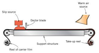
Figure 13.18 Schematic diagram showing the tape-casting process using a doctor blade. (From D. W. Richerson, *Modern Ceramic Engineering*, 2nd edition, Marcel Dekker, Inc., NY, 1992. Reprinted from *Modern Ceramic Engineering*, 2nd edition, p. 472 by courtesy of Marcel Dekker, Inc.)
