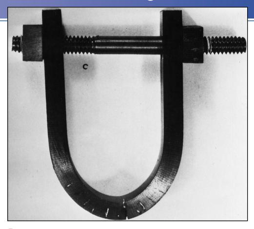
Photograph showing a bar of steel that has been bent into a "horseshoe" shape using a nut-andbolt assembly. While immersed in seawater, stress corrosion cracks formed along the bend at those regions where the tensile stresses are the greatest. (Photograph courtesy of F. L. LaQue. From F. L. LaQue, *Marine Corrosion, Causes and Prevention.* Copyright © 1975 by John Wiley & Sons, Inc. Reprinted by permission of John Wiley & Sons, Inc.)
