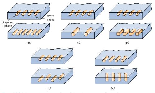
**Figure 16.1** Schematic representations of the various geometrical and spatial characteristics of particles of the dispersed phase that may influence the properties of composites: (*a*) concentration, (*b*) size, (*c*) shape, (*d*) distribution, and (*e*) orientation. (From Richard A. Flinn and Paul K. Trojan, *Engineering Materials and Their Applications*, 4th edition. Copyright © 1990 by John Wiley & Sons, Inc. Adapted by permission of John Wiley & Sons, Inc.)
