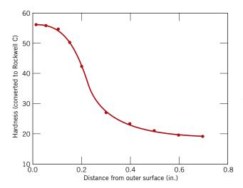
Figure 22.18 Transverse hardness profile across the axle cross section. (Microhardness readings were converted to Rockwell C values). [Reproduced with permission from *Handbook* of Case Studies in Failure Analysis, Vol. 1 (1992), ASM International, Materials Park, OH, 44073-0002.]
