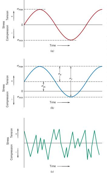
Figure 8.17 Variation of stress with time that accounts for fatigue failures. (a) Reversed stress cycle, in which the stress alternates from a maximum tensile stress (+) to a maximum compressive stress (-)of equal magnitude. (b) Repeated stress cycle, in which maximum and minimum stresses are asymmetrical relative to the zero-stress level; mean stress  $\sigma_m$ , range of stress  $\sigma_r$ , and stress amplitude  $\sigma_a$  are indicated. (c) Random stress cycle.
