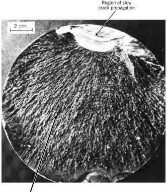
Figure 8.23 Fatigue failure surface. A crack formed at the top edge. The smooth region also near the top corresponds to the area over which the crack propagated slowly. Rapid failure occurred over the area having a dull and fibrous texture (the largest area). Approximately  $0.5 \times$ . [Reproduced by permission from *Metals* Handbook: Fractography and Atlas of Fractographs, Vol. 9, 8th edition, H. E. Boyer (Editor), American Society for Metals, 1974.]
