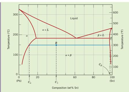
**Figure 9.9** The lead-tin phase diagram. For a 40 wt% Sn-60 wt% Pb alloy at  $150^{\circ}$ C (point *B*), phase compositions and relative amounts are computed in Example Problems 9.2 and 9.3.
