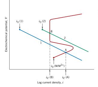
Figure 17.13 Demonstration of how an active–passive metal can exhibit both active and passive corrosion behaviors.
