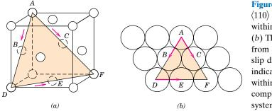
Figure 7.6 (a) A {111}  $\langle 110 \rangle$  slip system shown within an FCC unit cell. (b) The (111) plane from (a) and three  $\langle 110 \rangle$ slip directions (as indicated by arrows) within that plane comprise possible slip systems.
