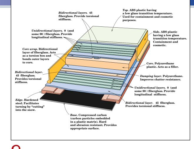
ne relatively complex composite structure is the modern ski. In this illustration, a cross section of a high-performance snow ski, are shown the various components. The function of each component is noted, as well as the material that is used in its construction. (Courtesy of Evolution Ski Company, Salt Lake City, Utah.)
