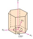
Figure 3.7 Coordinate axis system for a hexagonal unit cell (Miller–Bravais scheme).
