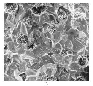
**Figure 8.6** (*a*) Schematic cross-section profile showing crack propagation through the interior of grains for transgranular fracture. (*b*) Scanning electron fractograph of ductile cast iron showing a transgranular fracture surface. Magnification unknown. [Figure (*b*) from V. J. Colangelo and F. A. Heiser, *Analysis of Metallurgical Failures*, 2nd edition. Copyright © 1987 by John Wiley & Sons, New York. Reprinted by permission of John Wiley & Sons, Inc.]
