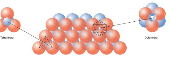
**Figure 12.7** The stacking of one plane of close-packed (orange) spheres (anions) on top of another (blue spheres); the geometries of tetrahedral and octahedral positions between the planes are noted. (From W. G. Moffatt, G. W. Pearsall, and J. Wulff, *The Structure and Properties of Materials*, Vol. I, *Structure*. Copyright © 1964 by John Wiley & Sons, New York. Reprinted by permission of John Wiley & Sons, Inc.)
