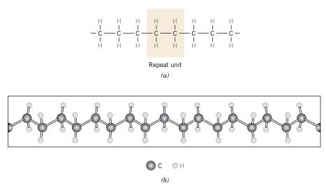
The polymer chain then forms by the sequential addition of monomer units to this active growing chain molecule. The active site, or unpaired electron (denoted by  $\cdot$ ), is transferred to each successive end monomer as it is linked to the chain. This may be represented schematically as follows:
