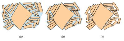
**Figure 13.13** Several stages in the removal of water from between clay particles during the drying process. (*a*) Wet body. (*b*) Partially dry body. (*c*) Completely dry body. (From W. D. Kingery, *Introduction to Ceramics*. Copyright © 1960 by John Wiley & Sons, New York. Reprinted by permission of John Wiley & Sons, Inc.)
