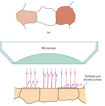
(a) Polished and etched grains as they might appear when viewed with an optical microscope. (b) Section taken through these grains showing how the etching characteristics and resulting surface texture vary from grain to grain because of differences in crystallographic orientation. (c) Photomicrograph of a polycrystalline brass specimen.  $60 \times$ . (Photomicrograph courtesy of J. E. Burke, General Electric Co.)
