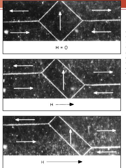
hotomicrographs of an iron single crystal, showing magnetic domains and their change in shape as a magnetic field (H) is applied. The magnetization direction of each domain is indicated by an arrow. Those domains that are favorably oriented with the applied field grow at the expense of the unfavorably oriented domains. (Photomicrographs courtesy of General Electric Research Laboratory.)
