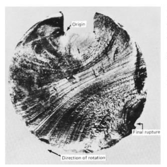
Figure 8.21 Fracture surface of a rotating steel shaft that experienced fatigue failure. Beachmark ridges are visible in the photograph. (Reproduced with permission from D. J. Wulpi, *Understanding How Components Fail*, American Society for Metals, Materials Park, OH, 1985.)
