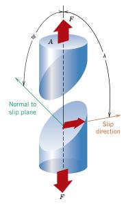
**Figure 7.7** Geometrical relationships between the tensile axis, slip plane, and slip direction used in calculating the resolved shear stress for a single crystal.
