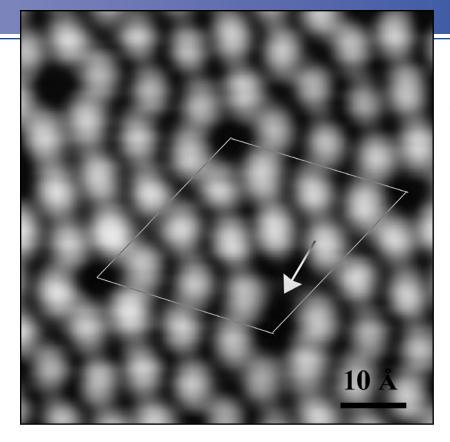
A scanning probe micrograph (generated using a scanning-tunneling microscope) that shows a (111)-type surface plane\* for silicon. The arrow points to the location of a silicon atom that was removed using a tungsten nanotip probe. This site from which an atom is missing is the surface analogue of a vacancy defect that is, a vacant lattice site within the bulk material. Approximately 20,000,000×. (Micrograph courtesy of D. Huang, Stanford University.)
