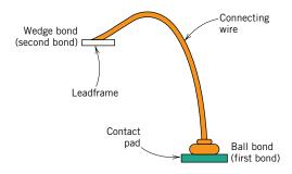
Figure 22.31 Schematic diagram showing a connecting wire that is ball bonded to the IC contact pad and wedge bonded to the leadframe. [Adapted from *Electronic Materials Handbook*, Vol. 1, *Packaging*, C. A. Dostal (Editor), ASM International, 1989, p. 225.]
