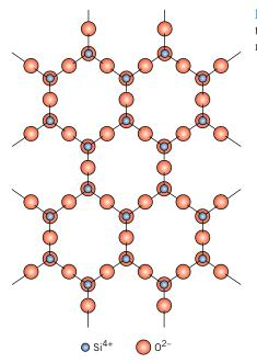
**Figure 12.13** Schematic representation of the two-dimensional silicate sheet structure having a repeat unit formula of  $(Si_2O_5)^{2^-}$ .
