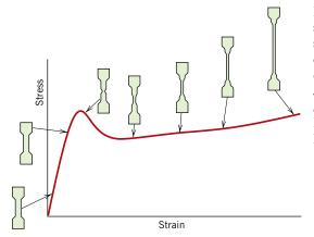
Figure 15.4 Schematic tensile stress-strain curve for a semicrystalline polymer. Specimen contours at several stages of deformation are included. (From Jerold M. Schultz, *Polymer Materials Science*, copyright © 1974, p. 488. Reprinted by permission of Prentice Hall, Inc., Englewood Cliffs, NJ.)
