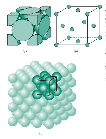
Figure 3.1 For the facecentered cubic crystal structure, (a) a hard sphere unit cell representation, (b) a reduced-sphere unit cell, and (c) an aggregate of many atoms. [Figure (c) adapted from W. G. Moffatt, G. W. Pearsall, and J. Wulff, The Structure and Properties of Materials, Vol. I, Structure, p. 51. Copyright © 1964 by John Wiley & Sons, New York. Reprinted by permission of John Wiley & Sons, Inc.]
