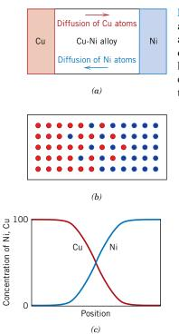
Figure 5.2 (a) A copper–nickel diffusion couple after a high-temperature heat treatment, showing the alloyed diffusion zone. (b) Schematic representations of Cu (red circles) and Ni (blue circles) atom locations within the couple. (c) Concentrations of copper and nickel as a function of position across the couple.
