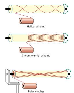
Figure 16.15 Schematic representations of helical, circumferential, and polar filament winding techniques. [From N. L. Hancox, (Editor), *Fibre Composite Hybrid Materials,* The Macmillan Company, New York, 1981.]
