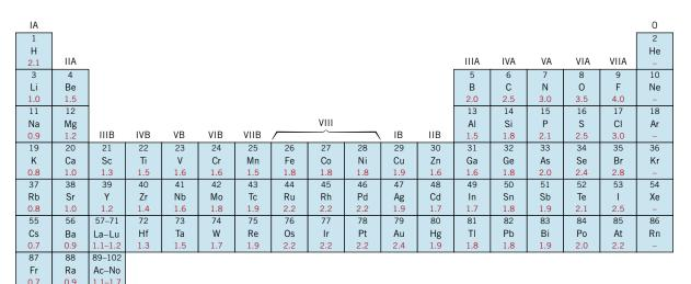
Figure 2.7 The electronegativity values for the elements. (Adapted from Linus Pauling, The Nature of the Chemical Bond, 3rd edition. Copyright 1939 and 1940, 3rd edition copyright © 1960, by Cornell University. Used by permission of the publisher, Cornell University Press.)
