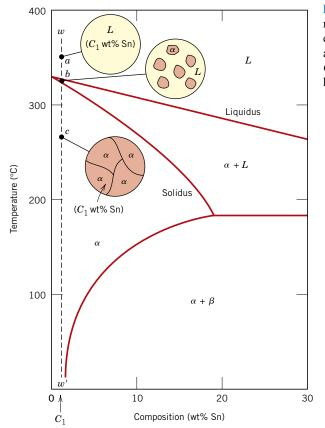
Figure 9.11 Schematic representations of the equilibrium microstructures for a lead-tin alloy of composition  $C_1$  as it is cooled from the liquid-phase region. upon cooling to room temperature. This microstructure is represented schematically by the inset at point c in Figure 9.11.
