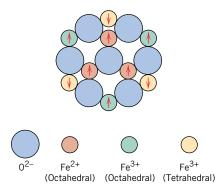
**Figure 20.9** Schematic diagram showing the spin magnetic moment configuration for  $Fe^{2+}$  and  $Fe^{3+}$  ions in  $Fe_3O_4$ . (From Richard A. Flinn and Paul K. Trojan, *Engineering Materials and Their Applications*, 4th edition. Copyright © 1990 by John Wiley & Sons, Inc. Adapted by permission of John Wiley & Sons, Inc.)
