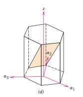
**3.50** Sketch the  $(01\overline{1}1)$  and  $(2\overline{11}0)$  planes in a hexagonal unit cell.
