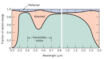
For example, cadmium sulfide (CdS) has a band gap of about 2.4 eV; hence, it absorbs photons having energies greater than about 2.4 eV, which correspond to the blue and violet portions of the visible spectrum; some of this energy is reradiated as light having other wavelengths. Nonabsorbed visible light consists of photons having energies between about 1.8 and 2.4 eV. Cadmium sulfide takes on a yellow-orange color because of the composition of the transmitted beam.
