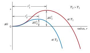
Figure 10.3 Schematic freeenergy-versus-embryo/nucleusradius curves for two different temperatures. The critical free energy change ( $\Delta G^*$ ) and critical nucleus radius ( $r^*$ ) are indicated for each temperature.
