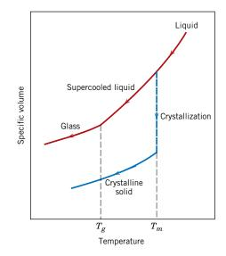
Figure 13.6 Contrast of specific volumeversus-temperature behavior of crystalline and noncrystalline materials. Crystalline materials solidify at the melting temperature  $T_m$ . Characteristic of the noncrystalline state is the glass transition temperature  $T_g$ .
