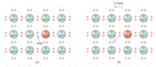
**Figure 18.14** Extrinsic *p*-type semiconduction model (electron bonding). (*a*) An impurity atom such as boron, having three valence electrons, may substitute for a silicon atom. This results in a deficiency of one valence electron, or a hole associated with the impurity atom. (*b*) The motion of this hole in response to an electric field.
