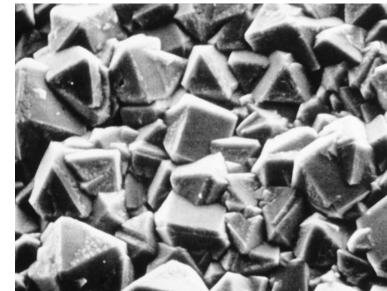
Figure 12.16 Scanning electron micrograph of a diamond thin film in which is shown numerous multifaceted microcrystals. 1000×. (Photograph courtesy of the Norton Company.)
