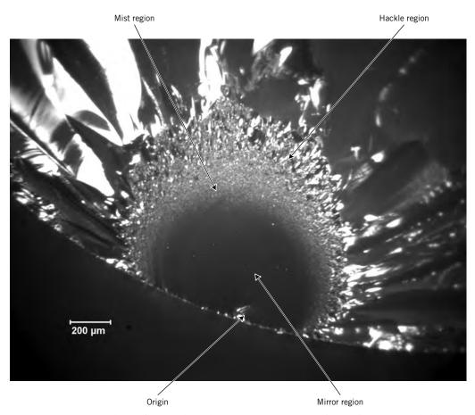
**Figure 12.31** Photomicrograph of the fracture surface of a 6 mm-diameter fused silica rod that was fractured in four-point bending. Features typical of this kind of fracture are noted—i.e., the origin, as well as mirror, mist, and hackle regions. 500×. (Courtesy of George Quinn, National Institute of Standards and Technology, Gaithersburg, MD.)
