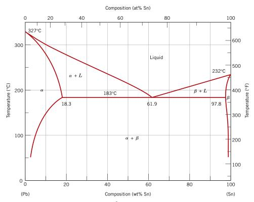
**Figure 9.8** The lead–tin phase diagram. [Adapted from *Binary Alloy Phase Diagrams*, 2nd edition, Vol. 3, T. B. Massalski (Editor-in-Chief), 1990. Reprinted by permission of ASM International, Materials Park, OH.]
