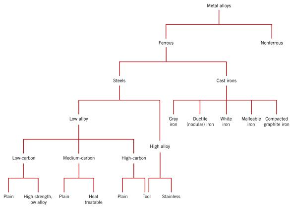
Figure 11.1 Classification scheme for the various ferrous alloys.
