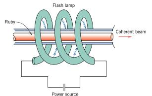
Figure 21.13 Schematic diagram of the ruby laser and xenon flash lamp. (From R. M. Rose, L. A. Shepard, and J. Wulff, *The Structure and Properties of Materials*, Vol. 4, *Electronic Properties*. Copyright © 1966 by John Wiley & Sons, New York. Reprinted by permission of John Wiley & Sons, Inc.)
