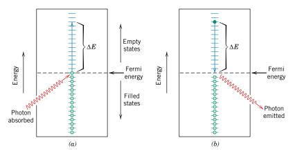
**Figure 21.4** (*a*) Schematic representation of the mechanism of photon absorption for metallic materials in which an electron is excited into a higher-energy unoccupied state. The change in energy of the electron  $\Delta E$  is equal to the energy of the photon. (*b*) Reemission of a photon of light by the direct transition of an electron from a high to a low energy state.
