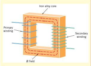
**Figure 20.20** Schematic diagram of a transformer core, including the direction of *B* field that is generated.
