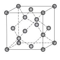
**Figure 12.15** A unit cell for the diamond cubic crystal structure.
