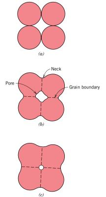
Figure 13.16 For a powder compact, microstructural changes that occur during firing. (*a*) Powder particles after pressing. (*b*) Particle coalescence and pore formation as sintering begins. (*c*) As sintering proceeds, the pores change size and shape.
