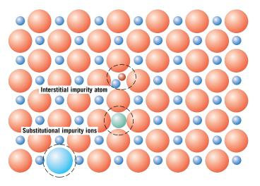
**Figure 12.23** Schematic representations of interstitial, anion-substitutional, and cationsubstitutional impurity atoms in an ionic compound. (Adapted from W. G. Moffatt, G. W. Pearsall, and J. Wulff, *The Structure and Properties of Materials*, Vol. I, *Structure*, p. 78. Copyright © 1964 by John Wiley & Sons, New York. Reprinted by permission of John Wiley & Sons, Inc.)
