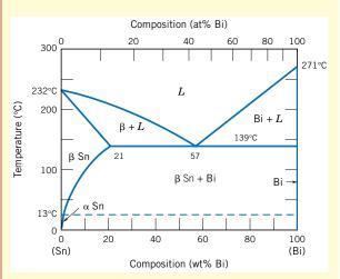
**Figure 9.10** The tin–bismuth phase diagram. [Adapted from *ASM Handbook*, Vol. 3, *Alloy Phase Diagrams*, H. Baker (Editor), ASM International, 1992, p. 2.106. Reprinted by permission of ASM International, Materials Park, OH.]
