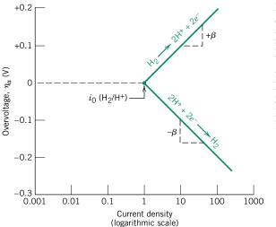
Figure 17.7 For a hydrogen electrode, plot of activation polarization overvoltage versus logarithm of current density for both oxidation and reduction reactions. (Adapted from M. G. Fontana, *Corrosion Engineering*, 3rd edition. Copyright © 1986 by McGraw-Hill Book Company. Reproduced with permission.)
