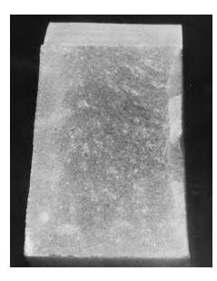
**Figure 22.19** Fracture surface of the Charpy impact specimen that was taken from the outer perimeter region. [Reproduced with permission from *Handbook of Case Studies in Failure Analysis, Vol. 1* (1992), ASM International, Materials Park, OH, 44073-0002.]
