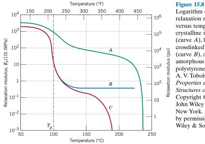
Logarithm of the relaxation modulus versus temperature for crystalline isotactic (curve A), lightly crosslinked atactic (curve B), and amorphous (curve C) polystyrene. (From A. V. Tobolsky, Properties and Structures of Polymers. Copyright © 1960 by John Wiley & Sons, New York. Reprinted by permission of John Wiley & Sons, Inc.)
