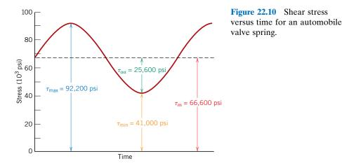
Now let us determine the actual stress amplitude  $\tau_{aa}$  for the valve spring using Equation 8.16 modified to the shear stress condition:
