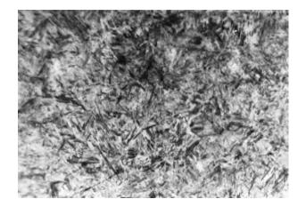
Figure 22.16 Optical photomicrograph of the failed axle outer perimeter region, which is composed of tempered martensite. 500×. [Reproduced with permission from *Handbook of Case Studies in Failure Analysis, Vol. 1* (1992), ASM International, Materials Park, OH, 44073-0002.]
