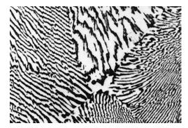
**Figure 9.14** Photomicrograph showing the microstructure of a lead–tin alloy of eutectic composition. This microstructure consists of alternating layers of a leadrich  $\alpha$ -phase solid solution (dark layers), and a tin-rich  $\beta$ -phase solid solution (light layers). 375×. (Reproduced with permission from *Metals Handbook*, 9th edition, Vol. 9, *Metallography and Microstructures*, American Society for Metals, Materials Park, OH, 1985.)
