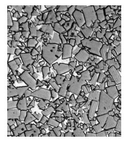
**Figure 16.4** Photomicrograph of a WC–Co cemented carbide. Light areas are the cobalt matrix; dark regions, the particles of tungsten carbide. 100×. (Courtesy of Carboloy Systems Department, General Electric Company.)
