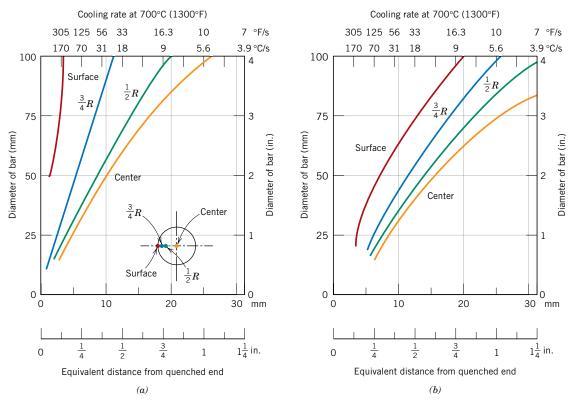
**Figure 11.17** Cooling rate as a function of diameter at surface, three-quarters radius  $(\frac{1}{4}R)$ , midradius  $(\frac{1}{2}R)$ , and center positions for cylindrical bars quenched in mildly agitated (*a*) water and (*b*) oil. Equivalent Jominy positions are included along the bottom axes. [Adapted from *Metals Handbook: Properties and Selection: Irons and Steels*, Vol. 1, 9th edition, B. Bardes (Editor), American Society for Metals, 1978, p. 492.]
