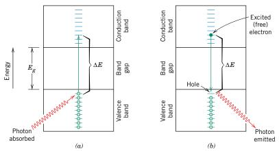
electron in the conduction band and a hole in the valence band are created. Again, the energy of excitation  $\Delta E$  is related to the absorbed photon frequency through Equation 21.6. These excitations with the accompanying absorption can take place only if the photon energy is greater than that of the band gap  $E_g$ —that is, if
