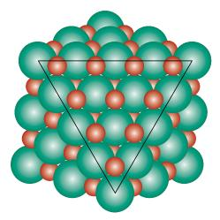
**Figure 12.8** A section of the rock salt crystal structure from which a corner has been removed. The exposed plane of anions (green spheres inside the triangle) is a {111}-type plane; the cations (red spheres) occupy the interstitial octahedral positions.
