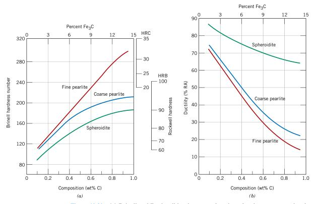
**Figure 10.30** (*a*) Brinell and Rockwell hardness as a function of carbon concentration for plain carbon steels having fine and coarse pearlite as well as spheroidite microstructures. (*b*) Ductility (%RA) as a function of carbon concentration for plain carbon steels having fine and coarse pearlite as well as spheroidite microstructures. (Data taken from *Metals Handbook: Heat Treating*, Vol. 4, 9th edition, V. Masseria, Managing Editor, American Society for Metals, 1981, pp. 9 and 17.)
