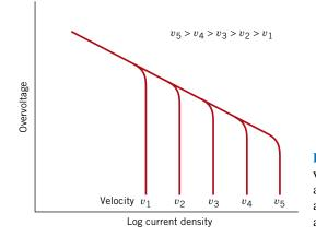
**Figure 17.26** Plot of overvoltage versus logarithm of current density for a solution that experiences combined activation–concentration polarization at various solution velocities.
