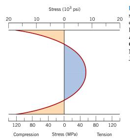
Figure 13.10 Room-temperature residual stress distribution over the cross section of a tempered glass plate. (From W. D. Kingery, H. K. Bowen, and D. R. Uhlmann, *Introduction to Ceramics*, 2nd edition. Copyright © 1976 by John Wiley & Sons, New York. Reprinted by permission of John Wiley & Sons, Inc.)
