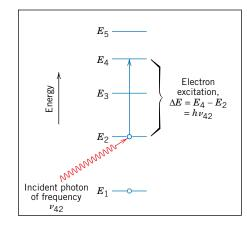
**Figure 21.3** For an isolated atom, a schematic illustration of photon absorption by the excitation of an electron from one energy state to another. The energy of the photon  $(h\nu_{42})$  must be exactly equal to the difference in energy between the two states  $(E_4 - E_2)$ .
