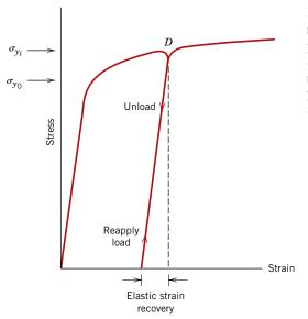
**Figure 6.17** Schematic tensile stress–strain diagram showing the phenomena of elastic strain recovery and strain hardening. The initial yield strength is designated as  $\sigma_{y_0}$ ;  $\sigma_{y_i}$  is the yield strength after releasing the load at point *D*, and then upon reloading.
