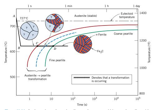
**Figure 10.14** Isothermal transformation diagram for a eutectoid iron–carbon alloy, with superimposed isothermal heat treatment curve (*ABCD*). Microstructures before, during, and after the austenite-to-pearlite transformation are shown. [Adapted from H. Boyer (Editor), *Atlas of Isothermal Transformation and Cooling Transformation Diagrams*, American Society for Metals, 1977, p. 28.]
