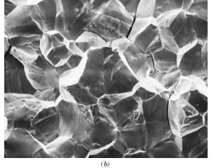
Figure 8.7 (a) Schematic cross-section profile showing crack propagation along grain boundaries for intergranular fracture. (b) Scanning electron fractograph showing an intergranular fracture surface.  $50 \times$ . [Figure (b) reproduced with permission from ASM Handbook, Vol. 12, Fractography, ASM International, Materials Park, OH, 1987.]
