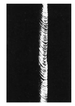
Figure 7.9 Slip in a zinc single crystal. (From C. F. Elam, *The Distortion of Metal Crystals*, Oxford University Press, London, 1935.)
