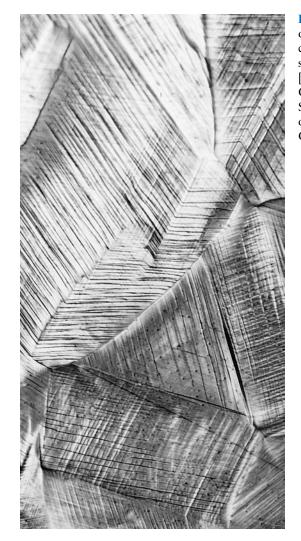
**Figure 7.10** Slip lines on the surface of a polycrystalline specimen of copper that was polished and subsequently deformed. 173×. [Photomicrograph courtesy of C. Brady, National Bureau of Standards (now the National Institute of Standards and Technology, Gaithersburg, MD).]
