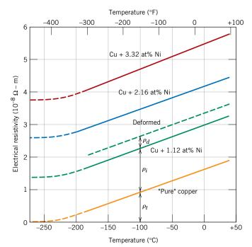
Figure 18.8 The electrical resistivity versus temperature for copper and three copper-nickel allovs, one of which has been deformed. Thermal, impurity, and deformation contributions to the resistivity are indicated at -100°C. [Adapted from J. O. Linde, Ann. Physik, 5, 219 (1932); and C.A. Wert and R. M. Thomson, Physics of Solids, 2nd edition, McGraw-Hill Book Company, New York, 1970.]
