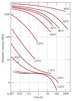
**Figure 15.27** Logarithm of relaxation modulus versus logarithm of time for poly(methyl methacrylate) between 40 and 135°C. (From J. R. McLoughlin and A. V. Tobolsky, *J. Colloid Sci.*, **7**, 555, 1952. Reprinted with permission.)
