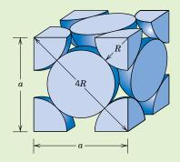
the atoms touch one another across a face-diagonal the length of which is 4R. Since the unit cell is a cube, its volume is  $a^3$ , where a is the cell edge length. From the right triangle on the face,
