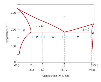
**Figure 9.18** The lead–tin phase diagram used in computations for relative amounts of primary  $\alpha$  and eutectic microconstituents for an alloy of composition  $C'_4$ .
