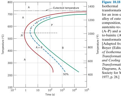
Isothermal transformation diagram for an iron-carbon alloy of eutectoid composition, including austenite-to-pearlite (A-P) and austeniteto-bainite (A-B) transformations. [Adapted from H. Boyer (Editor), Atlas of Isothermal **Transformation** and Cooling **Transformation** Diagrams, American Society for Metals, 1977, p. 28.]
