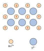
**Figure 20.8** Schematic representation of antiparallel alignment of spin magnetic moments for antiferromagnetic manganese oxide.
