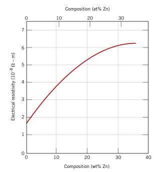
Figure 18.37 Room-temperature electrical resistivity versus composition for copper-zinc alloys. [Adapted from *Metals Handbook: Properties and Selection: Nonferrous Alloys and Pure Metals*, Vol. 2, 9th edition, H. Baker (Managing Editor), American Society for Metals, 1979, p. 315.]
