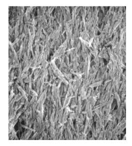
**Figure 20.24** A scanning electron micrograph showing the microstructure of a magnetic storage disk. Needle-shaped particles of  $\gamma$ -Fe<sub>2</sub>O<sub>3</sub> are oriented and embedded within an epoxy phenolic resin. 8000×. (Photograph courtesy of P. Rayner and N. L. Head, IBM Corporation.)
