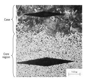
Figure 8.27 Photomicrograph showing both core (bottom) and carburized outer case (top) regions of a casehardened steel. The case is harder as attested by the smaller microhardness indentation.  $100 \times$ . (From R. W. Hertzberg, *Deformation and Fracture Mechanics of Engineering Materials*, 3rd edition. Copyright © 1989 by John Wiley & Sons, New York. Reprinted by permission of John Wiley & Sons, Inc.)
