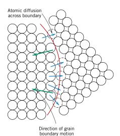
**Figure 7.24** Schematic representation of grain growth via atomic diffusion. (From Van Vlack, Lawrence H., *Elements of Materials Science and Engineering*, © 1989, p. 221. Adapted by permission of Pearson Education, Inc., Upper Saddle River, NJ.)
