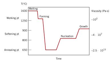
**Figure 13.11** Typical time-versus-temperature processing cycle for a Li<sub>2</sub>O–Al<sub>2</sub>O<sub>3</sub>–SiO<sub>2</sub> glass–ceramic. (Adapted from Y. M. Chiang, D. P. Birnie, III, and W. D. Kingery, *Physical Ceramics—Principles for Ceramic Science and Engineering*. Copyright © 1997 by John Wiley & Sons, New York. Reprinted by permission of John Wiley & Sons, Inc.)
