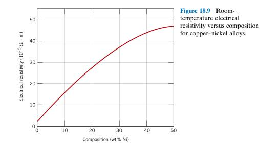
where A is a composition-independent constant that is a function of both the impurity and host metals. The influence of nickel impurity additions on the roomtemperature resistivity of copper is demonstrated in Figure 18.9, up to 50 wt% Ni; over this composition range nickel is completely soluble in copper (Figure 9.3*a*). Again, nickel atoms in copper act as scattering centers, and increasing the concentration of nickel in copper results in an enhancement of resistivity.
