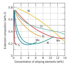
Figure 9.35 The dependence of eutectoid composition (wt% C) on alloy concentration for several alloying elements in steel. (From Edgar C. Bain, *Functions of the Alloying Elements in Steel*, American Society for Metals, 1939, p. 127.)
