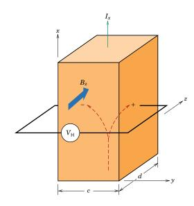
Figure 18.20 Schematic demonstration of the Hall effect. Positive and/or negative charge carriers that are part of the  $I_x$  current are deflected by the magnetic field  $B_z$  and give rise to the Hall voltage,  $V_{\rm H}$ . y direction. The magnitude of  $V_{\rm H}$  will depend on  $I_x$ ,  $B_z$ , and the specimen thickness d as follows:
