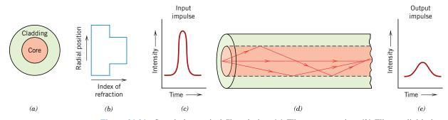
**Figure 21.21** Step-index optical fiber design. (*a*) Fiber cross section. (*b*) Fiber radial index of refraction profile. (*c*) Input light pulse. (*d*) Internal reflection of light rays. (*e*) Output light pulse. (Adapted from S. R. Nagel, *IEEE Communications Magazine*, Vol. 25, No. 4, p. 34, 1987.)
