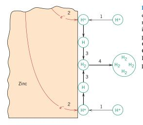
**Figure 17.6** Schematic representation of possible steps in the hydrogen reduction reaction, the rate of which is controlled by activation polarization. (From M. G. Fontana, *Corrosion Engineering,* 3rd edition. Copyright © 1986 by McGraw-Hill Book Company. Reproduced with permission.)
