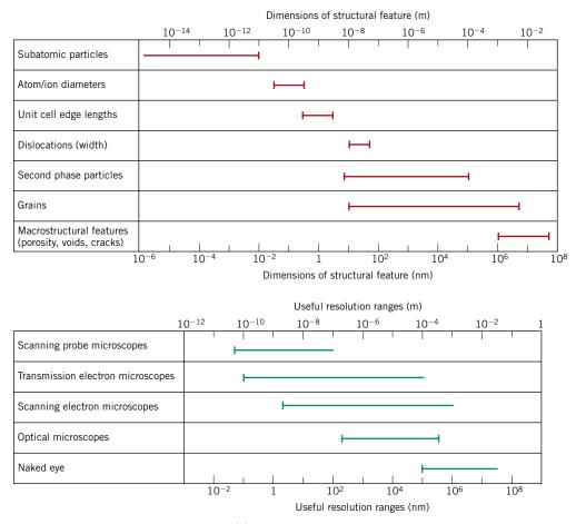
**Figure 4.15** (*a*) Bar-chart showing size ranges for several structural features found in materials. (*b*) Bar-chart showing the useful resolution ranges for four microscopic techniques discussed in this chapter, in addition to the naked eye. (Courtesy of Prof. Sidnei Paciornik, DCMM PUC-Rio, Rio de Janeiro, Brazil, and Prof. Carlos Pérez Bergmann, Federal University of Rio Grande do Sul, Porto Alegre, Brazil.)
