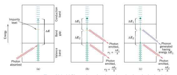
**Figure 21.6** (*a*) Photon absorption via a valence band-conduction band electron excitation for a material that has an impurity level that lies within the band gap. (*b*) Emission of two photons involving electron decay first into an impurity state, and finally to the ground state. (*c*) Generation of both a phonon and a photon as an excited electron falls first into an impurity level and finally back to its ground state.
