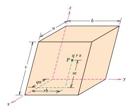
Figure 3.5 The manner in which the q, r, and s coordinates at point P within the unit cell are determined. The q coordinate (which is a fraction) corresponds to the distance qa along the x axis, where a is the unit cell edge length. The respective r and s coordinates for the y and z axes are determined similarly.
