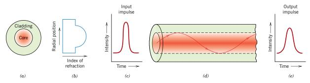
**Figure 21.22** Graded-index optical fiber design. (*a*) Fiber cross section. (*b*) Fiber radial index of refraction profile. (*c*) Input light pulse. (*d*) Internal reflection of a light ray. (*e*) Output light pulse. (Adapted from S. R. Nagel, *IEEE Communications Magazine*, Vol. 25, No. 4, p. 34, 1987.)
