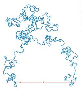
Figure 14.6 Schematic representation of a single polymer chain molecule that has numerous random kinks and coils produced by chain bond rotations. (From L. R. G. Treloar, *The Physics of Rubber Elasticity*, 2nd edition, Oxford University Press, Oxford, 1958, p. 47.)
