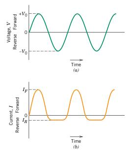
Figure 18.23 (a) Voltage versus time for the input to a p-n rectifying junction. (b) Current versus time, showing rectification of voltage in (a) by a p-nrectifying junction having the voltage-current characteristics shown in Figure 18.22.
