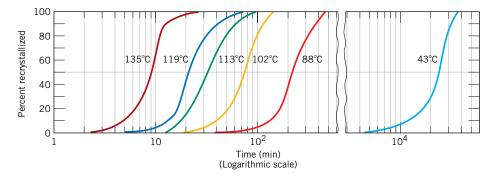
**Figure 10.11** Percent recrystallization as a function of time and at constant temperature for pure copper. (Reprinted with permission from *Metallurgical Transactions*, Vol. 188, 1950, a publication of The Metallurgical Society of AIME, Warrendale, PA. Adapted from B. F. Decker and D. Harker, "Recrystallization in Rolled Copper," *Trans. AIME*, **188**, 1950, p. 888.)
