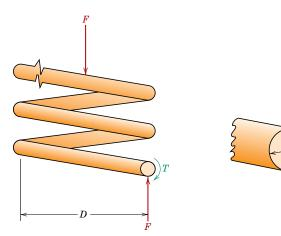
**Figure 22.4** Schematic diagram of a helical spring showing the twisting moment *T* that results from the compressive force *F*. (Adapted from K. Edwards and P. McKee, *Fundamentals of Mechanical Component Design*. Copyright © 1991 by McGraw-Hill, Inc. Reproduced with permission of The McGraw-Hill Companies.)
