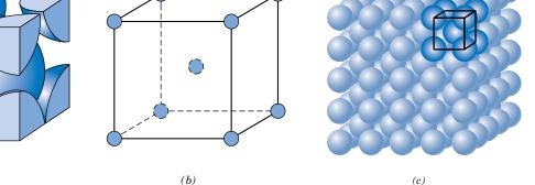
**Figure 3.2** For the body-centered cubic crystal structure, (*a*) a hard sphere unit cell representation, (*b*) a reduced-sphere unit cell, and (*c*) an aggregate of many atoms. [Figure (*c*) from W. G. Moffatt, G. W. Pearsall, and J. Wulff, *The Structure and Properties of Materials*, Vol. I, *Structure*, p. 51. Copyright © 1964 by John Wiley & Sons, New York. Reprinted by permission of John Wiley & Sons, Inc.]
