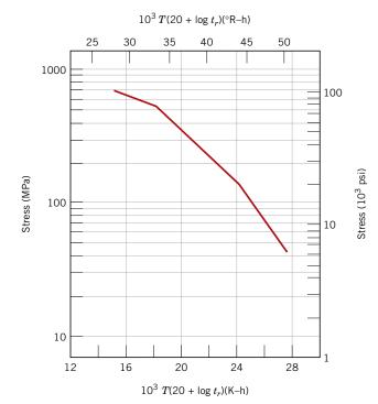
Figure 8.32 Logarithm stress versus the Larson–Miller parameter for an S-590 iron. (From F. R. Larson and J. Miller, *Trans. ASME*, 74, 765, 1952. Reprinted by permission of ASME.)
