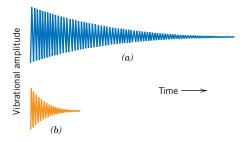
Figure 11.4 Comparison of the relative vibrational damping capacities of (*a*) steel and (*b*) gray cast iron. (From *Metals Engineering Quarterly*, February 1961. Copyright 1961 American Society for Metals.)
