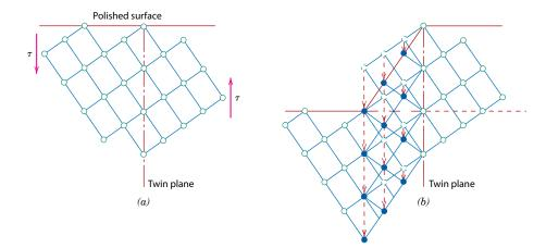
**Figure 7.12** Schematic diagram showing how twinning results from an applied shear stress  $\tau$ . In (*b*), open circles represent atoms that did not change position; dashed and solid circles represent original and final atom positions, respectively. (From G. E. Dieter, *Mechanical Metallurgy*, 3rd edition. Copyright © 1986 by McGraw-Hill Book Company, New York. Reproduced with permission of McGraw-Hill Book Company.)
