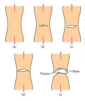
**Figure 8.2** Stages in the cup-and-cone fracture. (*a*) Initial necking. (*b*) Small cavity formation. (*c*) Coalescence of cavities to form a crack. (*d*) Crack propagation. (*e*) Final shear fracture at a 45° angle relative to the tensile direction. (From K. M. Ralls, T. H. Courtney, and J. Wulff, *Introduction to Materials Science and Engineering*, p. 468. Copyright © 1976 by John Wiley & Sons, New York. Reprinted by permission of John Wiley & Sons, Inc.)
