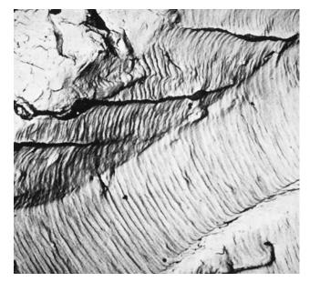
Figure 8.22 Transmission electron fractograph showing fatigue striations in aluminum. Magnification unknown. (From V. J. Colangelo and F. A. Heiser, *Analysis of Metallurgical Failures*, 2nd edition. Copyright © 1987 by John Wiley & Sons, New York. Reprinted by permission of John Wiley & Sons, Inc.)
