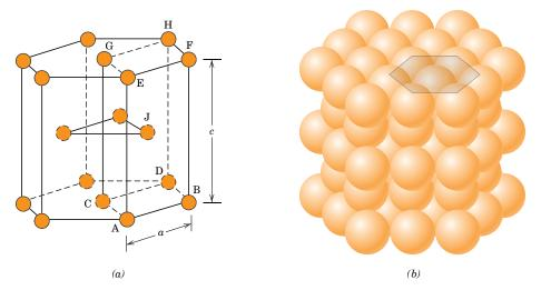
**Figure 3.3** For the hexagonal close-packed crystal structure, (*a*) a reduced-sphere unit cell (*a* and *c* represent the short and long edge lengths, respectively), and (*b*) an aggregate of many atoms. [Figure (*b*) from W. G. Moffatt, G. W. Pearsall, and J. Wulff, *The Structure and Properties of Materials*, Vol. I, *Structure*, p. 51. Copyright © 1964 by John Wiley & Sons, New York. Reprinted by permission of John Wiley & Sons, Inc.]
