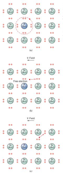
Figure 18.12 Extrinsic *n*-type semiconduction model (electron bonding). (*a*) An impurity atom such as phosphorus, having five valence electrons, may substitute for a silicon atom. This results in an extra bonding electron, which is bound to the impurity atom and orbits it. (*b*) Excitation to form a free electron. (*c*) The motion of this free electron in response to an electric field.
