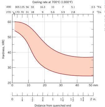
**Figure 11.16** The hardenability band for an 8640 steel indicating maximum and minimum limits. (Adapted from figure furnished courtesy Republic Steel Corporation.)
