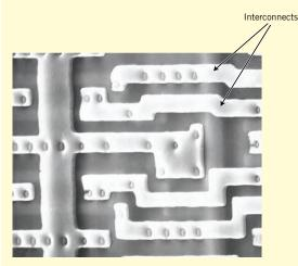
**Figure 5.9** Scanning electron micrograph of an integrated circuit chip, on which is noted aluminum interconnect regions. Approximately  $2000 \times$ . (Photograph courtesy of National Semiconductor Corporation.)
