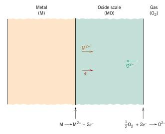
**Figure 17.24** Schematic representation of processes that are involved in gaseous oxidation at a metal surface.
