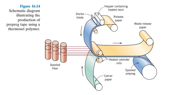
At room temperature the thermoset matrix undergoes curing reactions; therefore, the prepreg is stored at  $0^{\circ}C$  (32°F) or lower. Also, the time in use at room temperature (or "out-time") must be minimized. If properly handled, thermoset prepregs have a lifetime of at least six months and usually longer.
