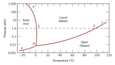
**Figure 9.2** Pressure–temperature phase diagram for H<sub>2</sub>O. Intersection of the dashed horizontal line at 1 atm pressure with the solid-liquid phase boundary (point 2) corresponds to the melting point at this pressure ( $T = 0^{\circ}$ C). Similarly, point 3, the intersection with the liquid-vapor boundary, represents the boiling point ( $T = 100^{\circ}$ C).
