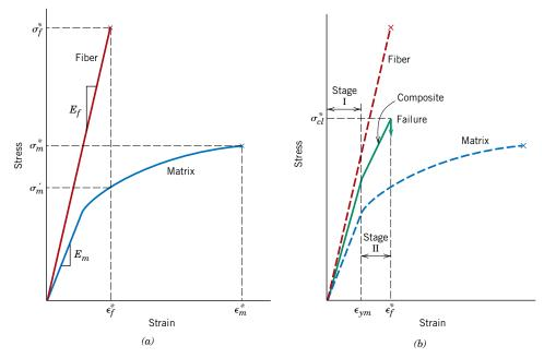
**Figure 16.9** (*a*) Schematic stress–strain curves for brittle fiber and ductile matrix materials. Fracture stresses and strains for both materials are noted. (*b*) Schematic stress–strain curve for an aligned fiber-reinforced composite that is exposed to a uniaxial stress applied in the direction of alignment; curves for the fiber and matrix materials shown in part (*a*) are also superimposed.
