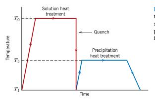
Figure 11.22 Schematic temperature-versus-time plot showing both solution and precipitation heat treatments for precipitation hardening.
