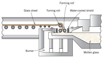
Figure 13.9 A process for the continuous drawing of sheet glass. (From W. D. Kingery, *Introduction to Ceramics*. Copyright © 1960 by John Wiley & Sons, New York. Reprinted by permission of John Wiley & Sons, Inc.)
