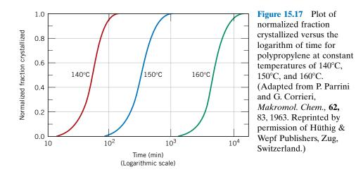
For polypropylene (as well as any polymer), the attainment of 100% crystallinity is not possible. Therefore, in Figure 15.17, the vertical axis is scaled as "normalized fraction crystallized." A value of 1.0 for this parameter corresponds to the highest level of crystallization that is achieved during the tests, which, in reality, is less than complete crystallization.
