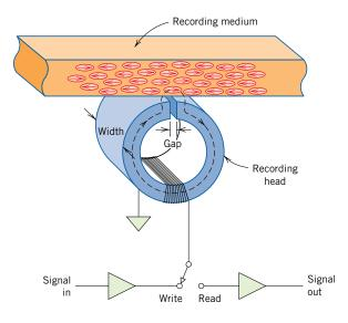
Figure 20.23 Schematic representation showing how information is stored and retrieved using a magnetic storage medium. (From J. U. Lemke, *MRS Bulletin*, Vol. XV, No. 3, p. 31, 1990. Reprinted with permission.)
