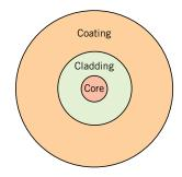
Figure 21.20 Schematic cross section of an optical fiber.
