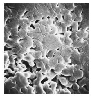
Figure 13.17 Scanning electron micrograph of an aluminum oxide powder compact that was sintered at 1700°C for 6 min. 5000×. (From W. D. Kingery, H. K. Bowen, and D. R. Uhlmann, *Introduction to Ceramics*, 2nd edition, p. 483. Copyright © 1976 by John Wiley & Sons, New York. Reprinted by permission of John Wiley & Sons, Inc.)
