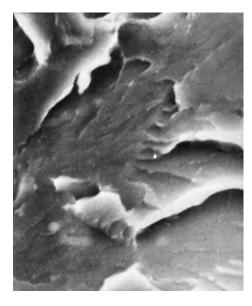
**Figure 22.14** Scanning electron micrograph of failed axle outer perimeter region near the keyway, which shows cleavage features.  $3500 \times$ . [Reproduced with permission from *Handbook of Case Studies in Failure Analysis, Vol. 1* (1992), ASM International, Materials Park, OH, 44073-0002.]
