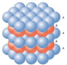
**Figure 3.14** Close-packed plane stacking sequence for hexagonal close-packed. (Adapted from W. G. Moffatt, G. W. Pearsall, and J. Wulff, *The Structure and Properties of Materials*, Vol. I, *Structure*, p. 51. Copyright © 1964 by John Wiley & Sons, New York. Reprinted by permission of John Wiley & Sons, Inc.)
