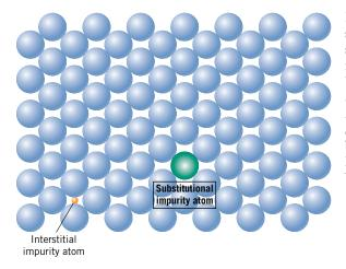
Figure 4.2 Two-dimensional schematic representations of substitutional and interstitial impurity atoms. (Adapted from W. G. Moffatt, G. W. Pearsall, and J. Wulff, *The Structure and Properties of Materials*, Vol. I, *Structure*, p. 77. Copyright © 1964 by John Wiley & Sons, New York. Reprinted by permission of John Wiley & Sons, Inc.)
