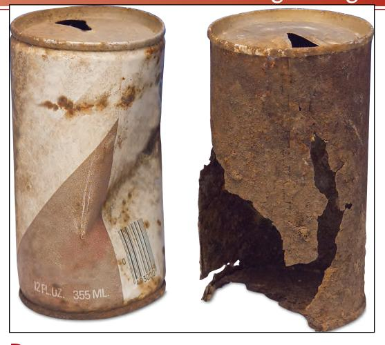
Photograph showing beverage cans that are made of an aluminum alloy (left) and a steel alloy (right). The steel beverage can has corroded significantly, and, therefore, is biodegradable and nonrecyclable. Conversely, the aluminum can is nonbiodegradable and recyclable inasmuch as it experienced very little corrosion.
