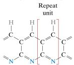
is so thermally stable that a woven cloth of this material can be heated directly in an open flame with no degradation. Polymers of this type are used in place of asbestos for high-temperature gloves.
