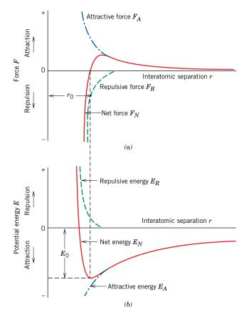
**Figure 2.8** (*a*) The dependence of repulsive, attractive, and net forces on interatomic separation for two isolated atoms. (*b*) The dependence of repulsive, attractive, and net potential energies on interatomic separation for two isolated atoms.
