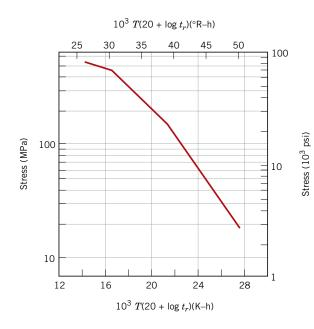
Figure 8.35 Logarithm stress versus the Larson–Miller parameter for an 18-8 Mo stainless steel. (From F. R. Larson and J. Miller, *Trans. ASME*, 74, 765, 1952. Reprinted by permission of ASME.)
