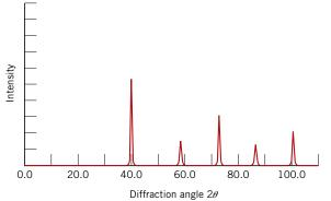
**Figure 3.24** Diffraction pattern for powdered tungsten. (Courtesy of Wesley L. Holman.)
