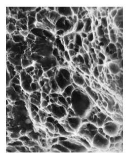
**Figure 22.23** Scanning electron micrograph of the fracture surface for the inner-core specimen that was tensile tested; a completely dimpled structure may be noted. Approximately 3500×. [Reproduced with permission from *Handbook of Case Studies in Failure Analysis, Vol. 1* (1992), ASM International, Materials Park, OH, 44073-0002.]
