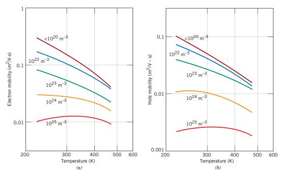
**Figure 18.19** Temperature dependence of (*a*) electron and (*b*) hole mobilities for silicon that has been doped with various donor and acceptor concentrations. Both sets of axes are scaled logarithmically. (From W. W. Gärtner, "Temperature Dependence of Junction Transistor Parameters," *Proc. of the IRE*, **45**, 667, 1957. Copyright © 1957 IRE now IEEE.)
