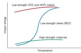
**Figure 8.15** Schematic curves for the three general types of impact energy-versus-temperature behavior.
