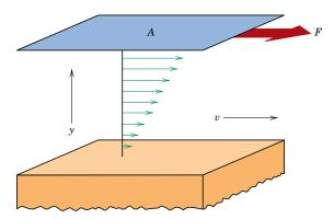
**Figure 12.34** Representation of the viscous flow of a liquid or fluid glass in response to an applied shear force.
