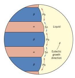
Figure 9.15 Schematic representation of the formation of the eutectic structure for the lead–tin system. Directions of diffusion of tin and lead atoms are indicated by blue and red arrows, respectively.
