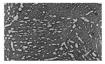
Figure 10.33 Electron micrograph of tempered martensite. Tempering was carried out at 594°C (1100°F). The small particles are the cementite phase; the matrix phase is  $\alpha$ -ferrite. 9300×. (Copyright 1971 by United States Steel Corporation.)
