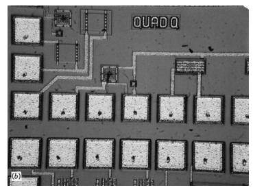
leadframe, which in turn is bonded to a printed circuit board. Enlarged photographs of microprocessor chips at different magnifications are presented in Figures 18.27*a* and 18.27*b*; these micrographs reveal the intricacy of integrated circuits. At this time, microprocessor chips approaching one billion transistors are being produced, and this number doubles about every 18 months.
