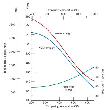
**Figure 10.34** Tensile and yield strengths and ductility (% RA) (at room temperature) versus tempering temperature for an oil-quenched alloy steel (type 4340). (Adapted from figure furnished courtesy Republic Steel Corporation.)
