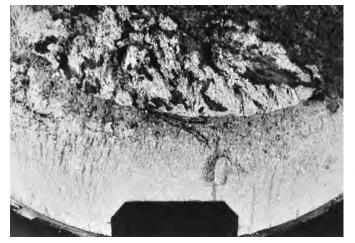
Figure 22.13 Optical micrograph of failed section of axle that shows the keyway (bottom), as well as the flat outer perimeter and rough core regions. [Reproduced with permission from *Handbook of Case Studies in Failure Analysis, Vol. 1* (1992), ASM International, Materials Park, OH, 44073-0002.]
