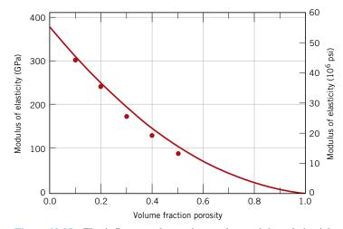
**Figure 12.35** The influence of porosity on the modulus of elasticity for aluminum oxide at room temperature. The curve drawn is according to Equation 12.9. (From R. L. Coble and W. D. Kingery, "Effect of Porosity on Physical Properties of Sintered Alumina," *J. Am. Ceram. Soc.*, **39**, 11, Nov. 1956, p. 381. Reprinted by permission of the American Ceramic Society.)
