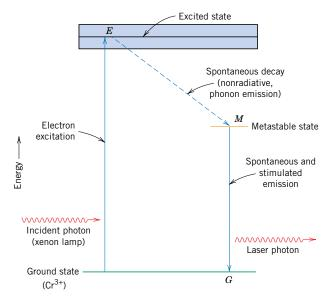
Figure 21.14 Schematic energy diagram for the ruby laser, showing electron excitation and decay paths.
