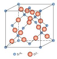
**Figure 12.10** The arrangement of silicon and oxygen atoms in a unit cell of cristobalite, a polymorph of SiO<sub>2</sub>.
