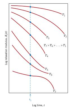
**Figure 15.6** Schematic plot of logarithm of relaxation modulus versus logarithm of time for a viscoelastic polymer; isothermal curves are generated at temperatures  $T_1$  through  $T_7$ . The temperature dependence of the relaxation modulus is represented as log  $E_r(t_1)$  versus temperature.
