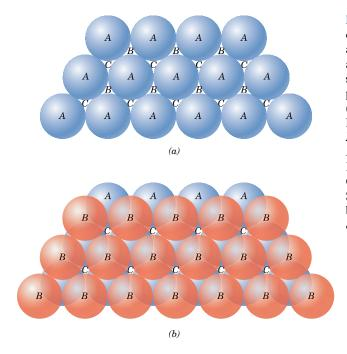
Figure 3.13 (a) A portion of a close-packed plane of atoms; A, B, and C positions are indicated. (b) The AB stacking sequence for closepacked atomic planes. (Adapted from W. G. Moffatt, G. W. Pearsall, and J. Wulff, The Structure and Properties of Materials, Vol. I, Structure, p. 50. Copyright © 1964 by John Wiley & Sons, New York. Reprinted by permission of John Wiley & Sons, Inc.)
