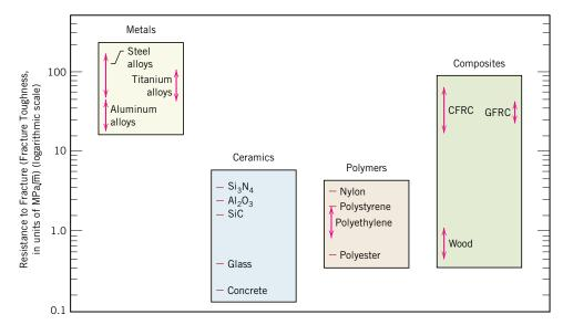
**Figure 1.6** Bar-chart of room-temperature resistance to fracture (i.e., fracture toughness) for various metals, ceramics, polymers, and composite materials. (Reprinted from *Engineering Materials 1: An Introduction to Properties, Applications and Design*, third edition, M. F. Ashby and D. R. H. Jones, pages 177 and 178, Copyright 2005, with permission from Elsevier.)
