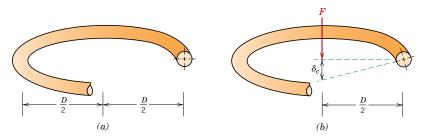
**Figure 22.5** Schematic diagrams of one coil of a helical spring, (*a*) prior to being compressed, and (*b*) showing the deflection  $\delta_c$  produced from the compressive force *F*. (Adapted from K. Edwards and P. McKee, *Fundamentals of Mechanical Component Design*. Copyright © 1991 by McGraw-Hill, Inc. Reproduced with permission of The McGraw-Hill Companies.)
