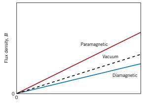
**Figure 20.6** Schematic representation of the flux density *B* versus the magnetic field strength *H* for diamagnetic and paramagnetic materials.
