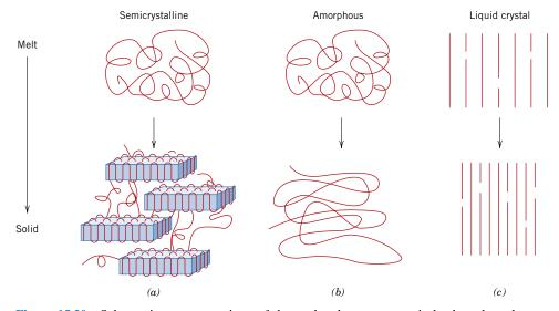
**Figure 15.20** Schematic representations of the molecular structures in both melt and solid states for (*a*) semicrystalline, (*b*) amorphous, and (*c*) liquid crystal polymers. (Adapted from G. W. Calundann and M. Jaffe, "Anisotropic Polymers, Their Synthesis and Properties," Chapter VII in *Proceedings of the Robert A. Welch Foundation Conferences on Polymer Research*, 26th Conference, Synthetic Polymers, Nov. 1982.)
