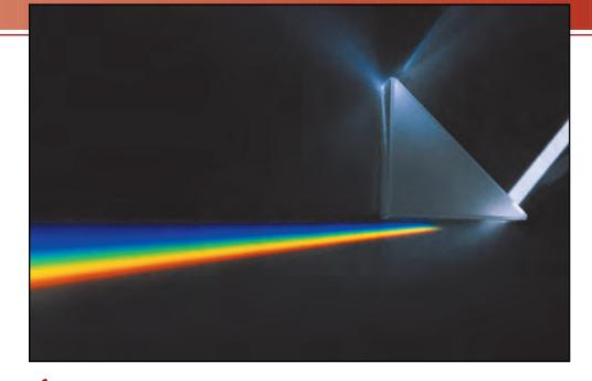
white light beam experiences both refraction and dispersion as it passes through the triangular glass prism. Refraction—in that the direction of the light beam is bent at both glass-air prism interfaces (i.e., as it passes into and out of the prism). And dispersion (chromatic)—in that the degree of bending depends on wavelength (i.e., the beam is separated into its component colors). (© PhotoDisc/Getty Images.)
