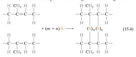
in which the two crosslinks shown consist of m and n sulfur atoms. Crosslink main chain sites are carbon atoms that were doubly bonded before vulcanization but, after vulcanization, have become singly bonded.
