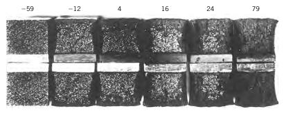
**Figure 8.14** Photograph of fracture surfaces of A36 steel Charpy V-notch specimens tested at indicated temperatures (in °C). (From R. W. Hertzberg, *Deformation and Fracture Mechanics of Engineering Materials,* 3rd edition, Fig. 9.6, p. 329. Copyright © 1989 by John Wiley & Sons, Inc., New York. Reprinted by permission of John Wiley & Sons, Inc.)
