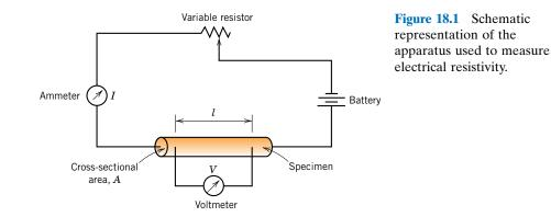
Electrical resistivity dependence on applied voltage, current, specimen cross-sectional area, and distance between measuring points
