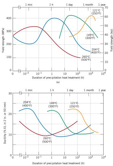
Figure 11.27 The precipitation hardening characteristics of a 2014 aluminum alloy (0.9 wt% Si, 4.4 wt% Cu, 0.8 wt% Mn, 0.5 wt% Mg) at four different aging temperatures: (a) vield strength, and (b) ductility (%EL). [Adapted from Metals Handbook: Properties and Selection: Nonferrous Alloys and Pure Metals, Vol. 2, 9th edition, H. Baker (Managing Editor), American Society for Metals, 1979, p. 41.]
