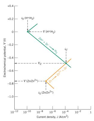
Figure 17.10 Electrode kinetic behavior of zinc in an acid solution; both oxidation and reduction reactions are rate limited by activation polarization. (Adapted from M. G. Fontana, *Corrosion Engineering*, 3rd edition. Copyright © 1986 by McGraw-Hill Book Company. Reproduced with permission.)
