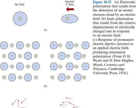
polarization that results from the distortion of an atomic electron cloud by an electric field. (b) Ionic polarization that results from the relative displacements of electrically charged ions in response to an electric field. (c) Response of permanent electric dipoles (arrows) to an applied electric field, producing orientation polarization. (From O. H. Wyatt and D. Dew-Hughes, Metals, Ceramics and Polymers, Cambridge University Press, 1974.)
