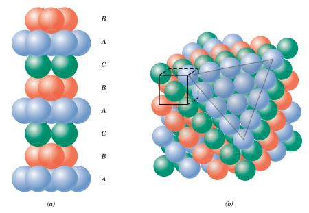
**Figure 3.15** (*a*) Close-packed stacking sequence for face-centered cubic. (*b*) A corner has been removed to show the relation between the stacking of close-packed planes of atoms and the FCC crystal structure; the heavy triangle outlines a (111) plane. [Figure (*b*) from W. G. Moffatt, G. W. Pearsall, and J. Wulff, *The Structure and Properties of Materials*, Vol. I, *Structure*, p. 51. Copyright © 1964 by John Wiley & Sons, New York. Reprinted by permission of John Wiley & Sons, Inc.]
