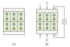
**Figure 18.36** (*a*) Dipoles within a piezoelectric material. (*b*) A voltage is generated when the material is subjected to a compressive stress. (From Van Vlack, Lawrence H., *Elements of Materials Science and Engineering*, © 1989, p. 482. Adapted by permission of Pearson Education, Inc., Upper Saddle River, New Jersey.)
