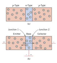
**Figure 18.25** For a junction transistor (p-n-p) type), the distributions and directions of electron and hole motion (a) when no potential is applied and (b) with appropriate bias for voltage amplification.
