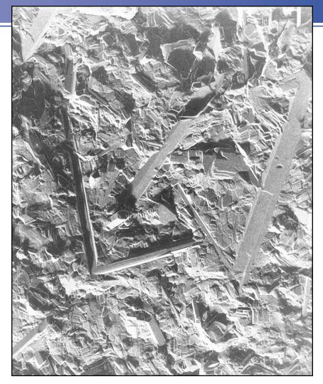
S canning electron micrograph showing the microstructure of a glass-ceramic material. The long acicular blade-shaped particles yield a material with unusual strength and toughness.  $65,000 \times$ . (Photograph courtesy of L. R. Pinckney and G. J. Fine of Corning Incorporated.)
