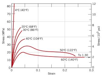
The influence of strain rate on the mechanical behavior may also be important. In general, decreasing the rate of deformation has the same influence on the stress-strain characteristics as increasing the temperature; that is, the material becomes softer and more ductile.
