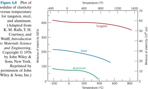
modulus of elasticity versus temperature for tungsten, steel, and aluminum. (Adapted from K. M. Ralls, T. H. Courtney, and J. Wulff, Introduction to Materials Science and Engineering. Copyright © 1976 by John Wiley & Sons, New York. Reprinted by permission of John Wiley & Sons, Inc.)
