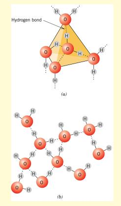
**Figure 2.16** The arrangement of water  $(H_2O)$  molecules in (*a*) solid ice, and (*b*) liquid water.
