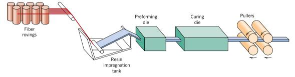
Figure 16.13 Schematic diagram showing the pultrusion process.
