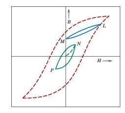
**Figure 20.15** A hysteresis curve at less than saturation (curve NP) within the saturation loop for a ferromagnetic material. The B-H behavior for field reversal at other than saturation is indicated by curve LM.
