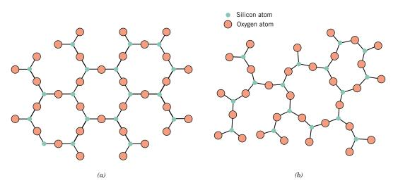
Figure 3.22 Two-dimensional schemes of the structure of (a) crystalline silicon dioxide and (b) noncrystalline silicon dioxide.
