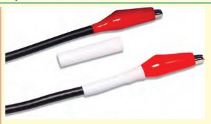
Photograph showing (from top to bottom) an electrical connection, a piece of as-received polymer shrink-tubing, and the constricted tubing around the junction—application of heat to the tubing caused its diameter to shrink. (Photography by S. Tanner.)
