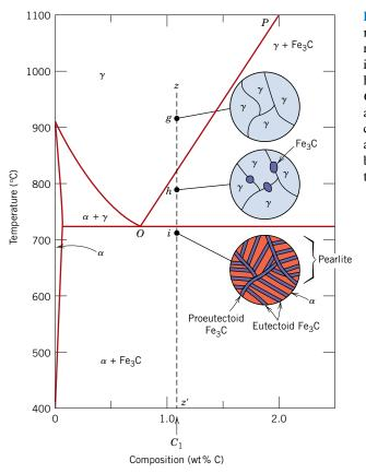
Figure 9.32 Schematic representations of the microstructures for an iron-carbon alloy of hypereutectoid composition  $C_1$  (containing between 0.76 and 2.14 wt% C), as it is cooled from within the austenite phase region to below the eutectoid temperature.
