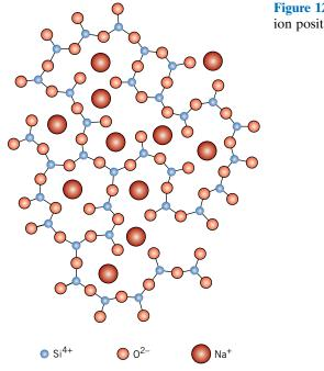
**Figure 12.11** Schematic representation of ion positions in a sodium–silicate glass.
