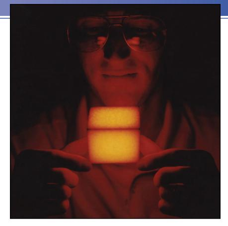
his photograph shows a whitehot cube of a silica fiber insulation material, which, only seconds after having been removed from a hot furnace, can be held by its edges with the bare hands. Initially, the heat transfer from the surface is relatively rapid; however, the thermal conductivity of this material is so small that heat conduction from the interior [maximum temperature approximately 1250°C (2300°F)] is extremely slow.
