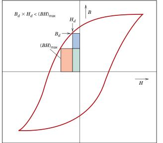
Figure 20.22 Schematic magnetization curve that displays hysteresis. Within the second quadrant are drawn two B-H energy product rectangles; the area of that rectangle labeled  $(BH)_{max}$  is the largest possible, which is greater than the area defined by  $B_d-H_d$ .
