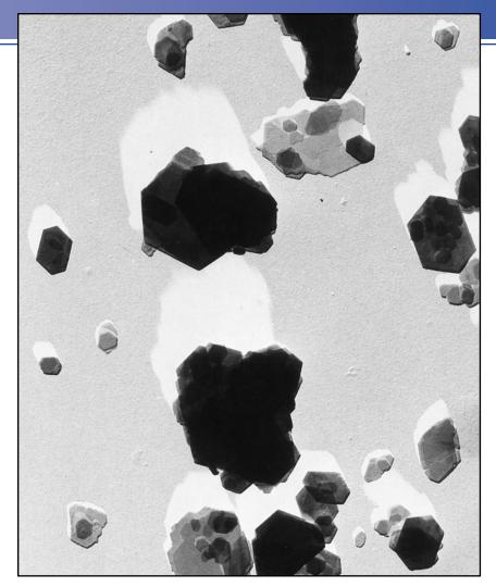
Electron micrograph of kaolinite crystals. They are in the form of hexagonal plates, some of which are stacked on top of one another. 21,000×. (Photograph courtesy of Georgia Kaolin Co., Inc.)
