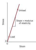
**Figure 6.5** Schematic stress–strain diagram showing linear elastic deformation for loading and unloading cycles.
