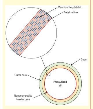
**Figure 16.19** Schematic diagram showing the crosssection of a high-performance Double  $Core^{TM}$  tennis ball. The inset drawing presents a detailed view of the nanocomposite coating that acts as a barrier to air permeation.
