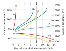
Figure 9.34 The dependence of eutectoid temperature on alloy concentration for several alloying elements in steel. (From Edgar C. Bain, *Functions of the Alloying Elements in Steel*, American Society for Metals, 1939, p. 127.)
