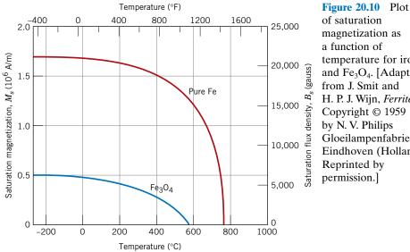
magnetization as a function of temperature for iron and Fe<sub>3</sub>O<sub>4</sub>. [Adapted from J. Smit and H. P. J. Wijn, Ferrites. Copyright © 1959 by N. V. Philips Gloeilampenfabrieken, Eindhoven (Holland). Reprinted by permission.]
