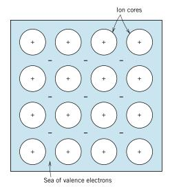
Figure 2.11 Schematic illustration of metallic bonding.
