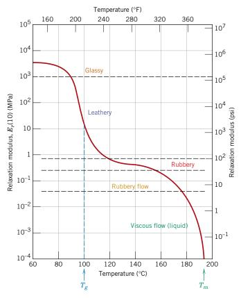
Figure 15.7 Logarithm of the relaxation modulus versus temperature for amorphous polystyrene, showing the five different regions of viscoelastic behavior. (From A. V. Tobolsky, *Properties and Structures of Polymers*. Copyright © 1960 by John Wiley & Sons, New York. Reprinted by permission of John Wiley & Sons, Inc.)
