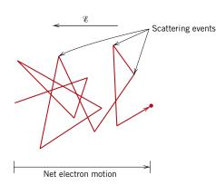
where *n* is the number of free or conducting electrons per unit volume (e.g., per cubic meter), and |e| is the absolute magnitude of the electrical charge on an electron  $(1.6 \times 10^{-19} \text{ C})$ . Thus, the electrical conductivity is proportional to both the number of free electrons and the electron mobility.
