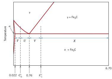
Figure 9.31 A portion of the Fe–Fe<sub>3</sub>C phase diagram used in computations for relative amounts of proeutectoid and pearlite microconstituents for hypoeutectoid  $(C'_0)$ and hypereutectoid  $(C'_1)$  compositions.
