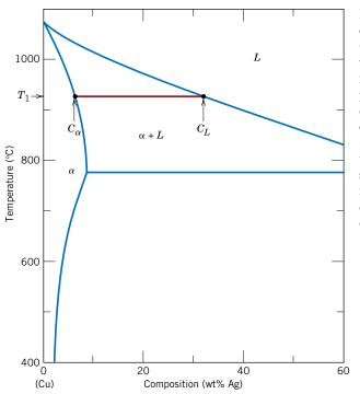
**Figure 9.23** Enlarged copper-rich section of the Cu–Ag phase diagram in which the Gibbs phase rule for the coexistence of two phases (i.e.,  $\alpha$  and L) is demonstrated. Once the composition of either phase (i.e.,  $C_{\alpha}$  or  $C_L$ ) or the temperature (i.e.,  $T_1$ ) is specified, values for the two remaining parameters are established by construction of the appropriate tie line.
