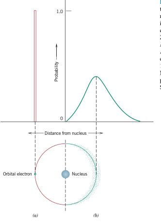
Figure 2.3 Comparison of the (*a*) Bohr and (*b*) wavemechanical atom models in terms of electron distribution. (Adapted from Z. D. Jastrzebski, *The Nature and Properties of Engineering Materials*, 3rd edition, p. 4. Copyright © 1987 by John Wiley & Sons, New York. Reprinted by permission of John Wiley & Sons, Inc.)
