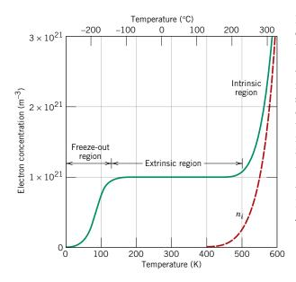
Figure 18.17 Electron concentration versus temperature for silicon (*n*-type) that has been doped with  $10^{21} \text{ m}^{-3}$  of a donor impurity, and for intrinsic silicon (dashed line). Freezeout, extrinsic, and intrinsic temperature regimes are noted on this plot. (From S. M. Sze, Semiconductor Devices, Physics and Technology. Copyright © 1985 by Bell Telephone Laboratories, Inc. Reprinted by permission of John Wiley & Sons, Inc.)
