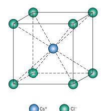
**Figure 12.3** A unit cell for the cesium chloride (CsCl) crystal structure.
