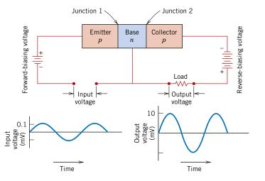
the load resistor, which is also shown in the circuit (Figure 18.24). Thus, a voltage signal that passes through a junction transistor experiences amplification; this effect is also illustrated in Figure 18.24 by the two voltage–time plots.
