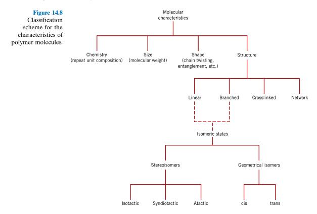
and network structures are all possible, in addition to several isomeric configurations (isotactic, syndiotactic, atactic, cis, and trans). These molecular characteristics are presented in the taxonomic chart, Figure 14.8. Note that some of the structural elements are not mutually exclusive of one another, and, in fact, it may be necessary to specify molecular structure in terms of more than one. For example, a linear polymer may also be isotactic.
