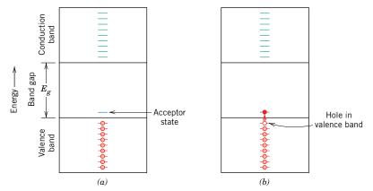
a hole in the valence band; a free electron is *not* created in either the impurity level or the conduction band. An impurity of this type is called an *acceptor*, because it is capable of accepting an electron from the valence band, leaving behind a hole. It follows that the energy level within the band gap introduced by this type of impurity is called an **acceptor state**.
