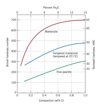
Figure 10.32 Hardness (at room temperature) as a function of carbon concentration for plain carbon martensitic, tempered martensitic [tempered at 371°C (700°F)], and pearlitic steels. (Adapted from Edgar C. Bain, *Functions of the Alloying Elements in Steel*, American Society for Metals, 1939, p. 36; and R. A. Grange, C. R. Hribal, and L. F. Porter, *Metall. Trans. A*, Vol. 8A, p. 1776.)
