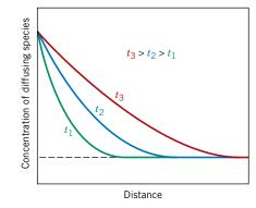
**Figure 5.5** Concentration profiles for nonsteady-state diffusion taken at three different times,  $t_1$ ,  $t_2$ , and  $t_3$ .
