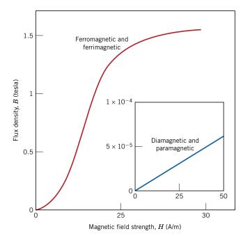
**Figure 20.16** Comparison of *B*-versus-*H* behaviors for ferromagnetic/ferrimagnetic and diamagnetic/ paramagnetic materials (inset plot). Here it may be noted that extremely small *B* fields are generated in materials that experience only diamagnetic/ paramagnetic behavior, which is why they are considered to be nonmagnetics.
