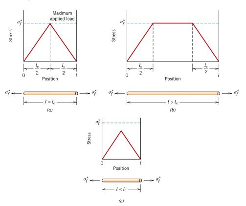
significantly less than  $l_c$ , the matrix deforms around the fiber such that there is virtually no stress transference and little reinforcement by the fiber. These are essentially the particulate composites as described above. To affect a significant improvement in strength of the composite, the fibers must be continuous.
