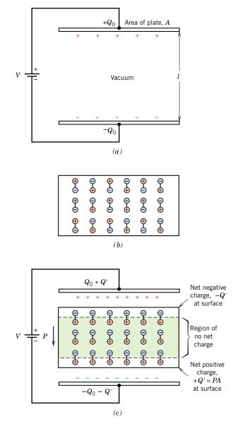
**Figure 18.31** Schematic representations of (*a*) the charge stored on capacitor plates for a vacuum, (*b*) the dipole arrangement in an unpolarized dielectric, and (*c*) the increased charge storing capacity resulting from the polarization of a dielectric material. (Adapted from A. G. Guy, *Essentials of Materials Science*, McGraw-Hill Book Company, New York, 1976.)
