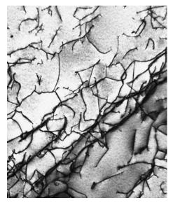
**Figure 4.6** A transmission electron micrograph of a titanium alloy in which the dark lines are dislocations. 51,450×. (Courtesy of M. R. Plichta, Michigan Technological University.)
