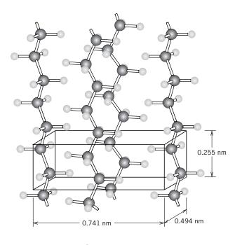
Figure 14.10 Arrangement of molecular chains in a unit cell for polyethylene. (Adapted from C. W. Bunn, *Chemical Crystallography*, Oxford University Press, Oxford, 1945, p. 233.)
