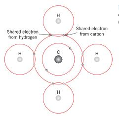
Figure 2.10 Schematic representation of covalent bonding in a molecule of methane  $(CH_4)$ .
