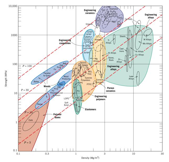
**Figure 22.2** Strength versus density materials selection chart. Design guidelines for performance indices of 3, 10, 30, and 100  $(MPa)^{2/3}m^3/Mg$  have been constructed, all having a slope of  $\frac{3}{2}$ . (Adapted from M. F. Ashby, *Materials Selection in Mechanical Design*. Copyright © 1992. Reprinted by permission of Butterworth-Heinemann Ltd.)
