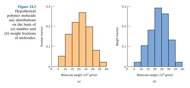
ranges and then determining the number fraction of chains within each size range (Figure 14.3*a*). The number-average molecular weight is expressed as
