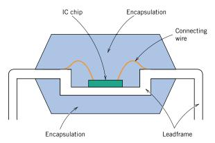
Figure 22.33 Schematic diagram showing an encapsulated IC leadframe package. [Adapted from *Electronic Materials Handbook*, Vol. 1. *Packaging*, C. A. Dostal (Editor), ASM International, 1989, p. 241.]
