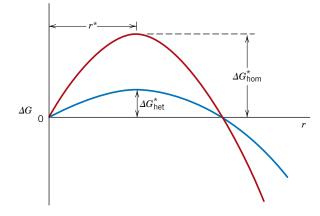
Figure 10.6 Schematic freeenergy-versus-embryo/nucleusradius plot on which are presented curves for both homogeneous and heterogeneous nucleation. Critical free energies and the critical radius are also shown.
