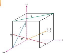
**3.32** Determine the indices for the directions shown in the following cubic unit cell:
