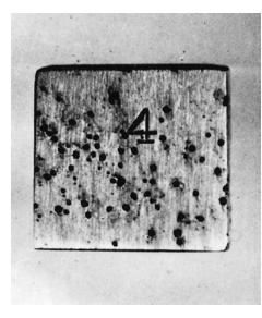
**Figure 17.17** The pitting of a 304 stainless steel plate by an acid-chloride solution. (Photograph courtesy of Mars G. Fontana. From M. G. Fontana, *Corrosion Engineering*, 3rd edition. Copyright © 1986 by McGraw-Hill Book Company. Reproduced with permission.)
