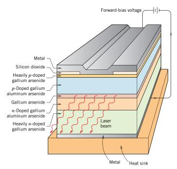
Figure 21.17 Schematic diagram showing the layered cross section of a GaAs semiconducting laser. Holes, excited electrons, and the laser beam are confined to the GaAs layer by the adjacent n- and p-type GaAlAs layers. (Adapted from "Photonic Materials," by J. M. Rowell. Copyright © 1986 by Scientific American, Inc. All rights reserved.)
