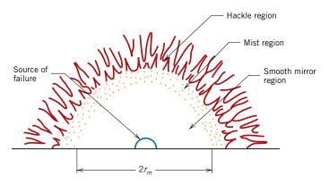
**Figure 12.30** Schematic diagram that shows typical features observed on the fracture surface of a brittle ceramic. (Adapted from J. J. Mecholsky, R. W. Rice, and S. W. Freiman, "Prediction of Fracture Energy and Flaw Size in Glasses from Measurements of Mirror Size," *J. Am. Ceram. Soc.*, **57** [10] 440 (1974). Reprinted with permission of The American Ceramic Society, *www.ceramics.org.* Copyright 1974. All rights reserved.)
