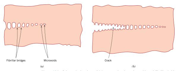
**Figure 15.9** Schematic drawings of (*a*) a craze showing microvoids and fibrillar bridges, and (*b*) a craze followed by a crack. (From J. W. S. Hearle, *Polymers and Their Properties*, Vol. 1, *Fundamentals of Structure and Mechanics*, Ellis Horwood, Ltd., Chichester, West Sussex, England, 1982.)
