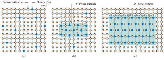
**Figure 11.25** Schematic depiction of several stages in the formation of the equilibrium precipitate ( $\theta$ ) phase. (*a*) A supersaturated  $\alpha$  solid solution. (*b*) A transition,  $\theta''$ , precipitate phase. (*c*) The equilibrium  $\theta$  phase, within the  $\alpha$ -matrix phase.
