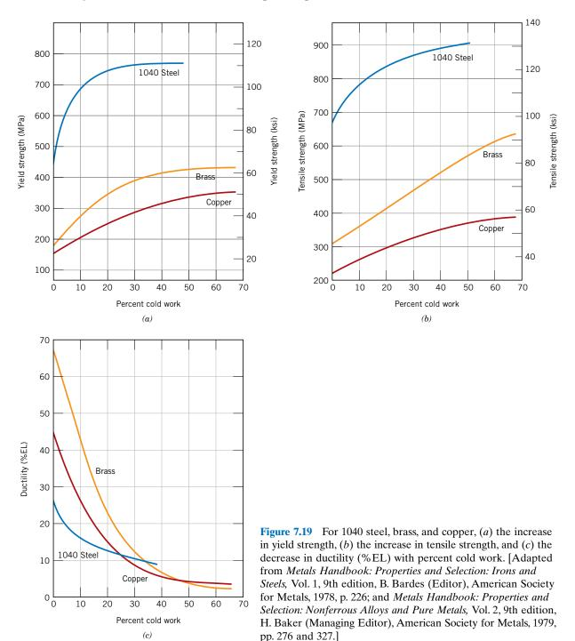
Figures 7.19*a* and 7.19*b* demonstrate how steel, brass, and copper increase in yield and tensile strength with increasing cold work. The price for this enhancement of hardness and strength is in the ductility of the metal. This is shown in Figure 7.19*c*, in which the ductility, in percent elongation, experiences a reduction with increasing percent cold work for the same three alloys. The influence of cold work on the
