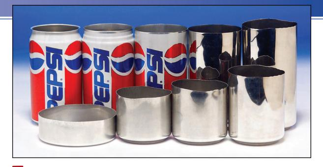
his photograph shows the aluminum beverage can in various stages of production. The can is formed from a single sheet of an aluminum alloy. Production operations include drawing, dome forming, trimming, cleaning, decorating, and neck and flange forming. (PEPSI is a registered trademark of PepsiCo, Inc. Used by permission.)
