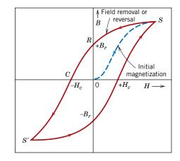
Figure 20.14 Magnetic flux density versus the magnetic field strength for a ferromagnetic material that is subjected to forward and reverse saturations (points *S* and *S'*). The hysteresis loop is represented by the solid curve; the dashed curve indicates the initial magnetization. The remanence  $B_r$  and the coercive force  $H_c$  are also shown.
