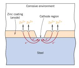
**Figure 17.23** Galvanic protection of steel as provided by a coating of zinc.
