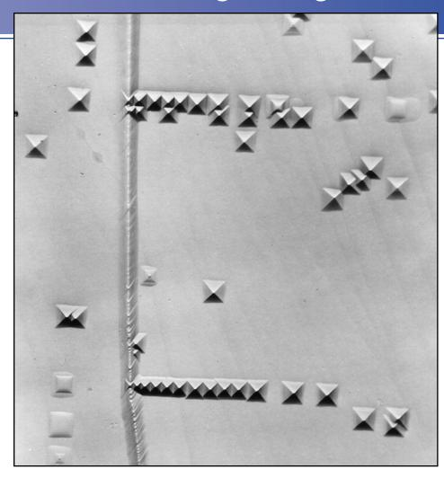
n this photomicrograph of a lithium fluoride (LiF) single crystal, the small pyramidal pits represent those positions at which dislocations intersect the surface. The surface was polished and then chemically treated; these "etch pits" result from localized chemical attack around the dislocations and indicate the distribution of the dislocations. 750×. (Photomicrograph courtesy of W. G. Johnston, General Electric Co.)
