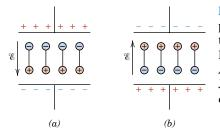
**Figure 18.33** Dipole orientations for (*a*) one polarity of an alternating electric field and (*b*) for the reversed polarity. (From Richard A. Flinn and Paul K. Trojan, *Engineering Materials and Their Applications*, 4th edition. Copyright © 1990 by John Wiley & Sons, Inc. Adapted by permission of John Wiley & Sons, Inc.)
