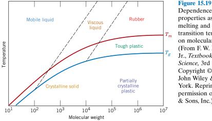
Dependence of polymer properties as well as melting and glass transition temperatures on molecular weight. (From F. W. Billmeyer, Jr., *Textbook of Polymer Science*, 3rd edition. Copyright © 1984 by John Wiley & Sons, New York. Reprinted by permission of John Wiley & Sons, Inc.)
