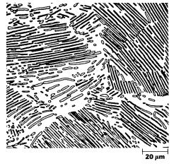
**Figure 9.27** Photomicrograph of a eutectoid steel showing the pearlite microstructure consisting of alternating layers of  $\alpha$  ferrite (the light phase) and Fe<sub>3</sub>C (thin layers most of which appear dark). 500×. (Reproduced with permission from *Metals Handbook*, 9th edition, Vol. 9, *Metallography and Microstructures*, American Society for Metals, Materials Park, OH, 1985.)
