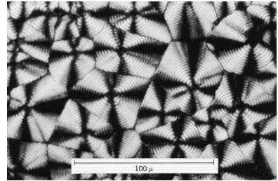
amorphous material. Tie-chain molecules that act as connecting links between adjacent lamellae pass through these amorphous regions.
