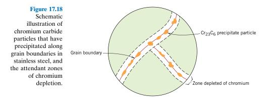
Intergranular corrosion is an especially severe problem in the welding of stainless steels, when it is often termed **weld decay.** Figure 17.19 shows this type of intergranular corrosion.
