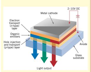
**Figure 21.12** Schematic diagram that shows the components and configuration of an organic light-emitting diode (OLED). (Reproduced by arrangement with *Silicon Chip* magazine.)
