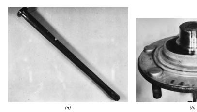
**Figure 22.12** (*a*) Photograph of one section of the failed axle. (*b*) Photograph showing wheel mounting flange and stub end of failed axle. [Reproduced with permission from *Handbook of Case Studies in Failure Analysis, Vol. 1* (1992), ASM International, Materials Park, OH, 44073-0002.]
