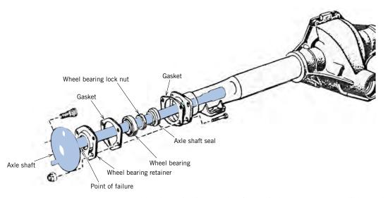
**Figure 22.11** Schematic diagram showing typical components of a light truck axle, and the fracture site for the failed axle of this case study. (Reproduced from *MOTOR Auto Repair Manual*, 39th Edition © Copyright 1975. By permission of the Hearst Corporation.)
