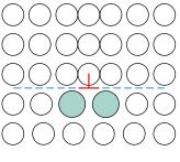
Figure 7.18 (a) Representation of compressive strains imposed on host atoms by a larger substitutional impurity atom. (b) Possible locations of larger impurity atoms relative to an edge dislocation such that there is partial cancellation of impurity–dislocation lattice strains.
