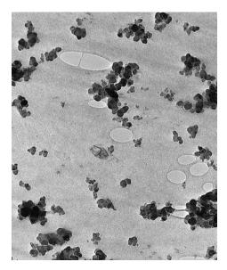
**Figure 16.5** Electron micrograph showing the spherical reinforcing carbon black particles in a synthetic rubber tire tread compound. The areas resembling water marks are tiny air pockets in the rubber.  $80,000 \times$ . (Courtesy of Goodyear Tire & Rubber Company.)
