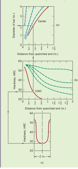
**Figure 11.19** Use of hardenability data in the generation of hardness profiles. (*a*) The cooling rate at the center of a water-quenched 50 mm (2 in.) diameter specimen is determined. (*b*) The cooling rate is converted into an HRC hardness for a 1040 steel. (*c*) The Rockwell hardness is plotted on the radial hardness profile.
