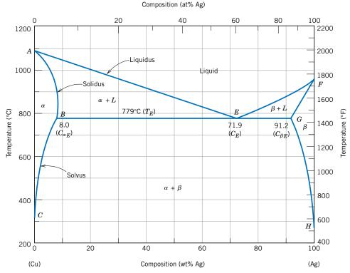
**Figure 9.7** The copper–silver phase diagram. [Adapted from *Binary Alloy Phase Diagrams*, 2nd edition, Vol. 1, T. B. Massalski (Editor-in-Chief), 1990. Reprinted by permission of ASM International, Materials Park, OH.]
