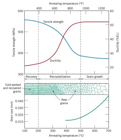
influence of annealing temperature (for an annealing time of 1 h) on the tensile strength and ductility of a brass alloy. Grain size as a function of annealing temperature is indicated. Grain structures during recovery, recrystallization, and grain growth stages are shown schematically. (Adapted from G. Sachs and K. R. Van Horn, Practical Metallurgy, Applied Metallurgy and the Industrial Processing of Ferrous and Nonferrous Metals and Alloys, American Society for Metals, 1940, p. 139.)
