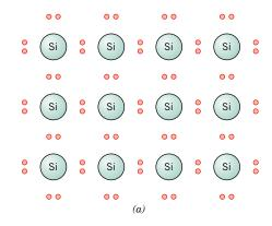
**Figure 18.11** Electron bonding model of electrical conduction in intrinsic silicon: (*a*) before excitation, (*b*) and (*c*) after excitation (the subsequent free-electron and hole motions in response to an external electric field).
