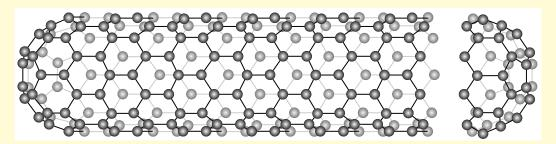
**Figure 12.19** The structure of a carbon nanotube. (Reprinted by permission from *American Scientist*, magazine of Sigma Xi, The Scientific Research Society. Illustration by Aaron Cox/*American Scientist*.)
