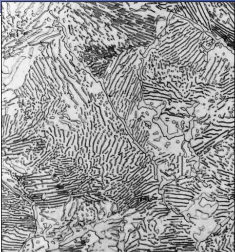
A photomicrograph of a pearlitic steel that has partially transformed to spheroidite. 2000×. (Courtesy of United States Steel Corporation.)
