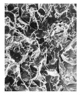
**Figure 22.15** Scanning electron micrograph of the failed axle rough central core region, which is composed of mixed cleavage and dimpled regions. 570×. [Reproduced with permission from *Handbook of Case Studies in Failure Analysis, Vol. 1* (1992), ASM International, Materials Park, OH, 44073-0002.]
