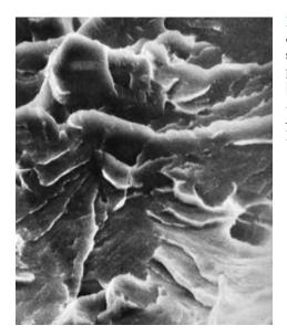
**Figure 22.21** Scanning electron micrograph of the fracture surface for the impact specimen prepared from the outer perimeter region of the failed axle. 3000×. [Reproduced with permission from *Handbook of Case Studies in Failure Analysis, Vol. 1* (1992), ASM International, Materials Park, OH, 44073-0002.]
