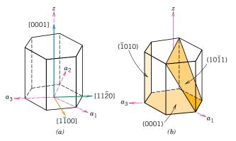
Figure 3.8 For the hexagonal crystal system, (a) [0001], [1 $\overline{1}$ 00], and [11 $\overline{2}$ 0] directions, and (b) the (0001), (10 $\overline{1}$ 1), and ( $\overline{1}$ 010) planes.
