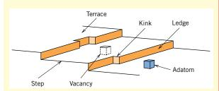
**Figure 4.10** Schematic representations of surface defects that are potential adsorption sites for catalysis. Individual atom sites are represented as cubes. (From BOUDART, MICHEL, *KINETICS OF HETEROGENEOUS CATALYTIC REACTIONS*. © 1984 Princeton University Press. Reprinted by permission of Princeton University Press.)
