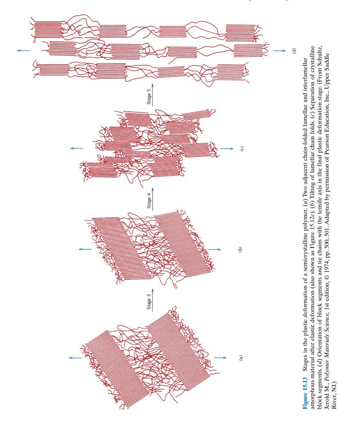
chains in the lamellae slide past one another (Figure 15.13*b*); this results in tilting of the lamellae so that the chain folds become more aligned with the tensile axis. Any chain displacement is resisted by relatively weak secondary or van der Waals bonds.
