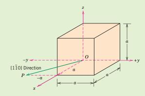
This problem is solved by reversing the procedure of the preceding example. For this [110] direction, the projections along the x, y, and z axes are a, -a, and 0a, respectively. This direction is defined by a vector passing from the origin to point P, which is located by first moving along the x axis a units, and from this position, parallel to the y axis -a units, as indicated in the figure. There is no z component to the vector, since the z projection is zero.
