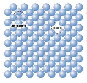
Figure 4.1 Two-dimensional representations of a vacancy and a self-interstitial. (Adapted from W. G. Moffatt, G. W. Pearsall, and J. Wulff, *The Structure and Properties of Materials*, Vol. I, *Structure*, p. 77. Copyright © 1964 by John Wiley & Sons, New York. Reprinted by permission of John Wiley & Sons, Inc.)
