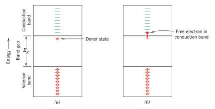
level is shifted upward in the band gap, to within the vicinity of the donor state; its exact position is a function of both temperature and donor concentration.
