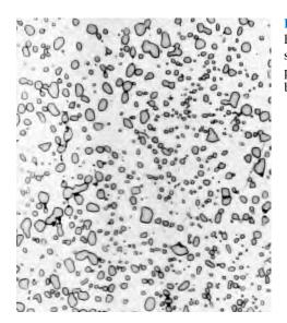
Figure 10.19 Photomicrograph of a steel having a spheroidite microstructure. The small particles are cementite; the continuous phase is  $\alpha$  ferrite. 1000×. (Copyright 1971 by United States Steel Corporation.)
