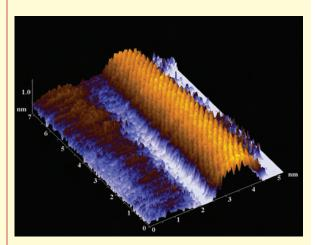
An atomically resolved image of a carbon nanotube that was generated using a scanning tunneling microscope (a type of scanning probe microscope, Section 4.10). Note the dimensional scales (in the nanometer range) along the sides of the micrograph. (Micrograph courtesy of Vladimir K. Nevolin, Moscow Institute of Electronic Engineering.)
