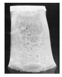
**Figure 22.20** Fracture surface of the Charpy impact specimen that was taken from the central core region. [Reproduced with permission from *Handbook of Case Studies in Failure Analysis, Vol. 1* (1992), ASM International, Materials Park, OH, 44073-0002.]
