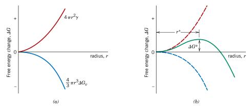
**Figure 10.2** (*a*) Schematic curves for volume free energy and surface free energy contributions to the total free energy change attending the formation of a spherical embryo/nucleus during solidification. (*b*) Schematic plot of free energy versus embryo/nucleus radius, on which is shown the critical free energy change ( $\Delta G^*$ ) and the critical nucleus radius ( $r^*$ ).
