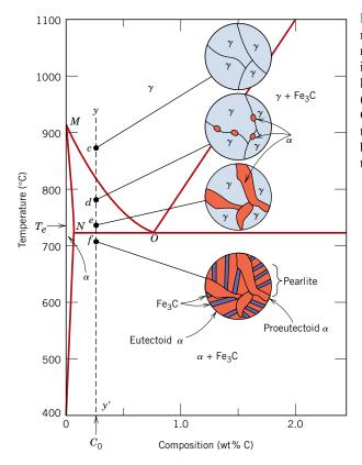
**Figure 9.29** Schematic representations of the microstructures for an iron–carbon alloy of hypoeutectoid composition  $C_0$  (containing less than 0.76 wt% C) as it is cooled from within the austenite phase region to below the eutectoid temperature.
