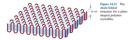
illustrated schematically in Figure 14.12. Each platelet will consist of a number of molecules; however, the average chain length will be much greater than the thickness of the platelet.
