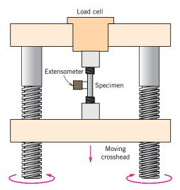
**Figure 6.3** Schematic representation of the apparatus used to conduct tensile stress-strain tests. The specimen is elongated by the moving crosshead; load cell and extensometer measure, respectively, the magnitude of the applied load and the elongation. (Adapted from H. W. Hayden, W. G. Moffatt, and J. Wulff, *The Structure and Properties of Materials*, Vol. III, *Mechanical Behavior*, p. 2. Copyright © 1965 by John Wiley & Sons, New York. Reprinted by permission of John Wiley & Sons, Inc.)
