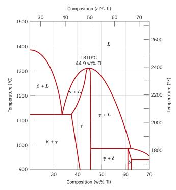
Figure 9.22 A portion of the nickel-titanium phase diagram on which is shown a congruent melting point for the  $\gamma$ -phase solid solution at 1310°C and 44.9 wt% Ti. [Adapted from *Phase Diagrams of Binary Nickel Alloys*, P. Nash (Editor), 1991. Reprinted by permission of ASM International, Materials Park, OH.]
