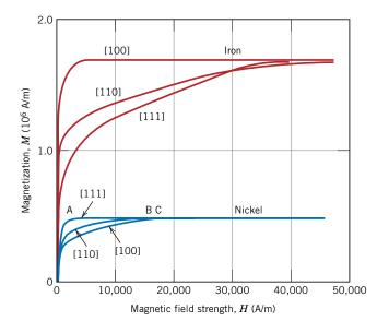
Figure 20.17 Magnetization curves for single crystals of iron and nickel. For both metals, a different curve was generated when the magnetic field was applied in each of [100], [110], and [111] crystallographic directions. [Adapted from K. Honda and S. Kaya, "On the Magnetisation of Single Crystals of Iron," Sci. Rep. Tohoku Univ., 15, 721 (1926); and from S. Kaya, "On the Magnetisation of Single Crystals of Nickel," Sci. Rep. Tohoku Univ., 17, 639 (1928).]
