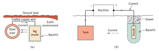
**Figure 17.22** Cathodic protection of (*a*) an underground pipeline using a magnesium sacrificial anode, and (*b*) an underground tank using an impressed current. (From M. G. Fontana, *Corrosion Engineering*, 3rd edition. Copyright © 1986 by McGraw-Hill Book Company. Reproduced with permission.)
