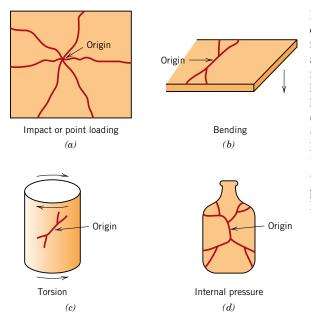
Figure 12.29 For brittle ceramic materials, schematic representations of crack origins and configurations that result from (*a*) impact (point contact) loading, (*b*) bending, (*c*) torsional loading, and (*d*) internal pressure. (From D. W. Richerson, *Modern Ceramic Engineering*, 2nd edition, Marcel Dekker, Inc., New York, 1992. Reprinted from *Modern Ceramic Engineering*, 2nd edition, p. 681, by courtesy of Marcel Dekker, Inc.)
